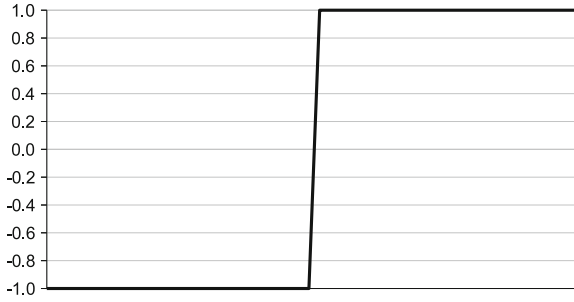
Fig. 1 SignumActivator ( mode = BIPOLAR, zeroValue = 0)
