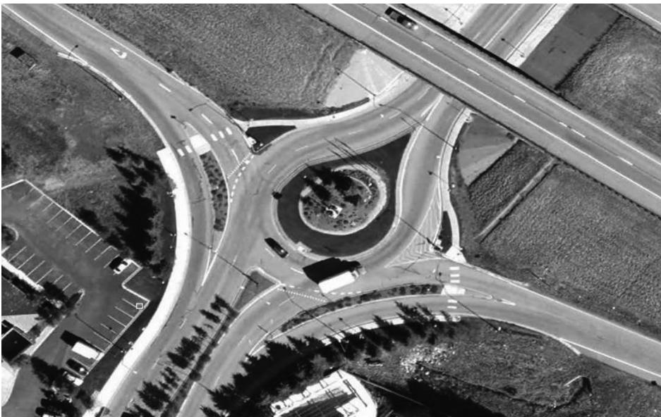
Figure 11.16 Teardrop crossing road ramp terminal. (From Leisch JP. Service interchange forms: Adaptability, design features and operational characteristics . Transportation System Planning, Boise, 2002.)
