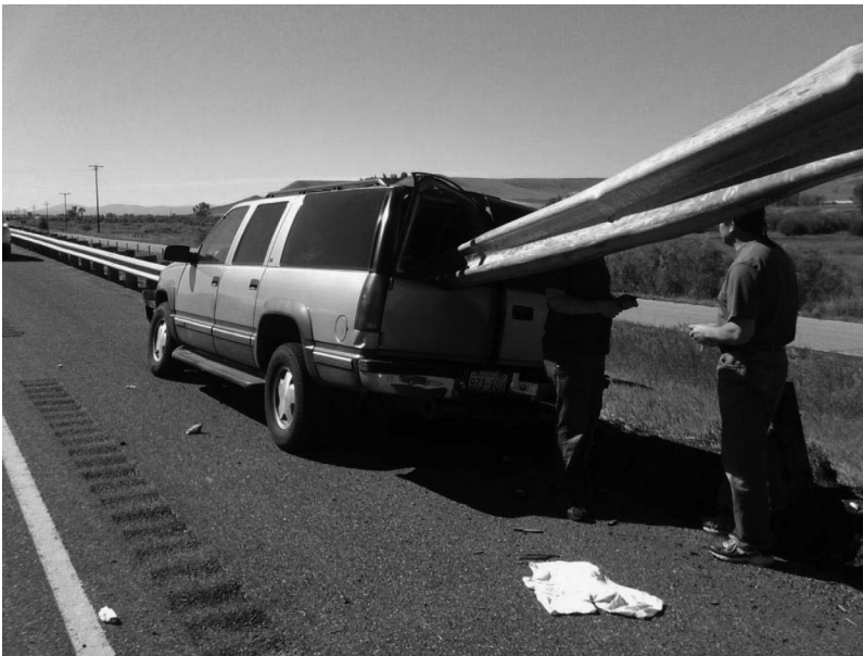
Figure 13.10 Vehicle impaled by guardrail terminal.
