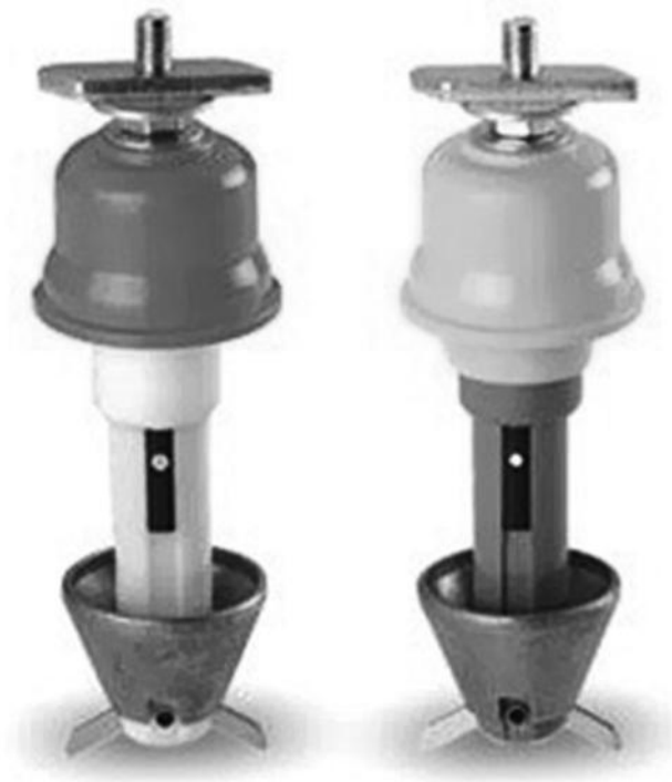
FIGURE 7.2 Ring frame creel—bobbin holders.
