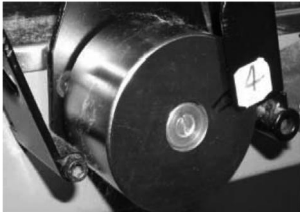
FIGURE 1.10 Sticky deposits on the draw frame creel.
