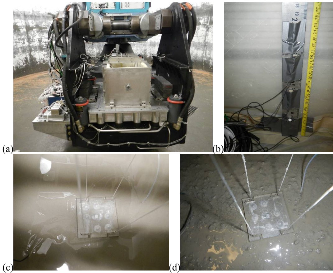
FIG. 2. (a) Laminar container bolted on shaker attached to the centrifuge basket, (b) Pore pressure sensors taped on ruler attached to the wall of the container and measuring tape used to monitor settlement, (c) Sensor glued on plastic plate floating on surface of mine tailings and (d) same sensor on surface of 2:1 mixture.
