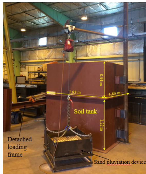
FIG. 1. Test setup and sand pluviation device
