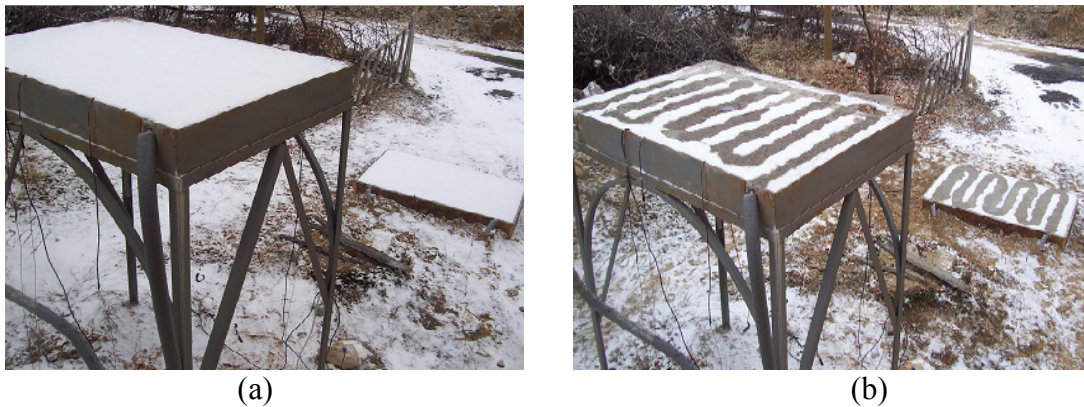
FIG. 3. Photographs of initial and intermediate snow melting process on slabs: (a) initial state ( t=0 ), (b) intermediate state ( t=30 min) (Balbay and Esen, 2010).
