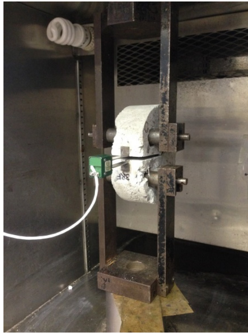
FIG. 3. DCT Fracture Test Setup
