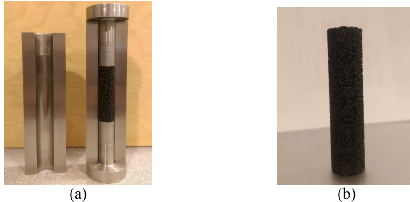
Fig 2. (a) Cylindrical mold to make FAM specimens, (b) FAM specimens.
