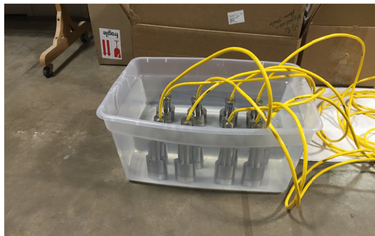
FIG. 2. Calibration test setup for VW piezometers
