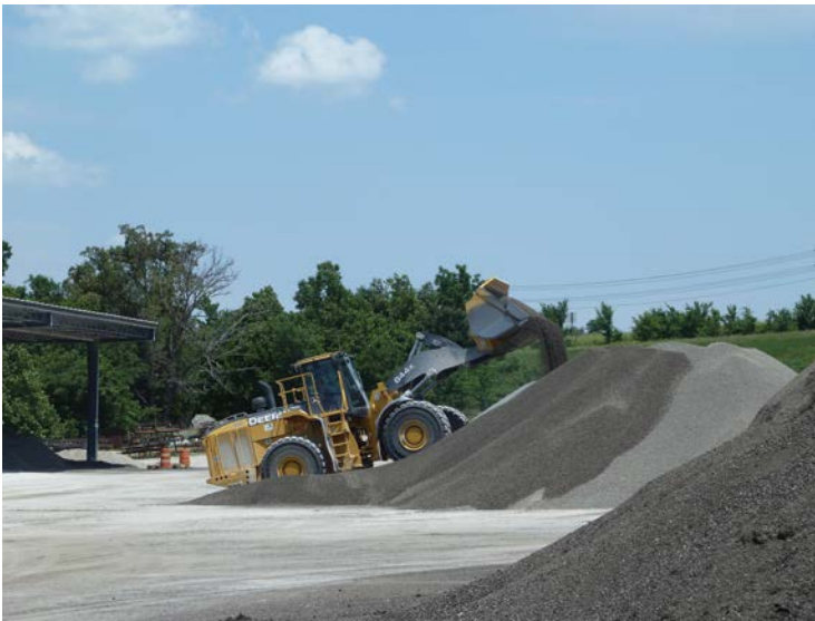
FIGURE 8.1 A stockpile of RAP in northwest Arkansas. (Credit: A. Braham.)
