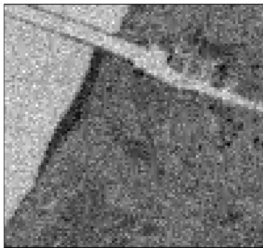
Figure 7.31 The magnitude of the adjusted norms of residual vectors represented by shades of gray (darker means larger values) for the AVIRIS image discussed in Example 7.11. As many as k = 100 principal components were used.
