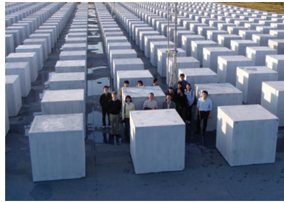
Figure 3.22 A one-fifth scale outdoor physical model, built as part of the Comprehensive Outdoor Scale Model Experiment (COSMO) on the campus of the Nippon Institute of Technology, Saitama Prefecture, Japan. The model (both base and cubes) is built from concrete coated with dark gray paint to provide identical radiative and thermal properties. The 512 cubes are approximately 1.5 m high, have a wall thickness of 0.1 m and have a plan area fraction \lambda_b = 0.25 . An 11 m high measurement tower is located in the centre of the array (Credit: M. Kanda and A. Inagaki; with permission). See Kanda and Moriizumi, (2009) for example results.
