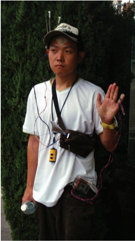
Figure 14.11 An outdoor Lagrangian measurement system suitable for evaluating the biometeorological environment. The antennae attached to the hat measure radiation, air temperature and humidity and wind speed; the instruments attached to the skin surfaces record skin temperature and heart rate and; the data-loggers recording the ambient environment and thermophysical responses are attached to the body (Credit: M. Nakayoshi; with permission).
