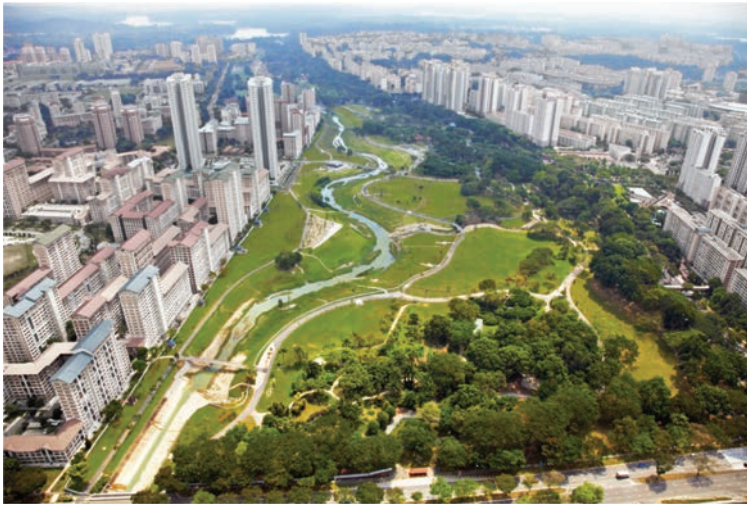
Figure 15.26 Aerial view of Bishan Park, Singapore, which was redesigned to increase the capacity of the Kallang River to cope with runoff from the urbanized landscape (Credit: Atelierdreiseitl; CC3.0).
