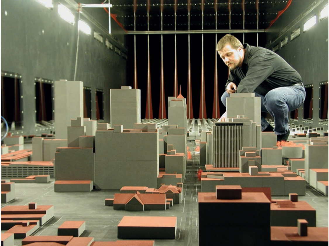
Figure 3.1 Physical scale model of central area of Oklahoma City, United States, in a wind tunnel illustrating that the geometric similarity of building shapes is preserved (Credit: B. Leitl; with permission).
