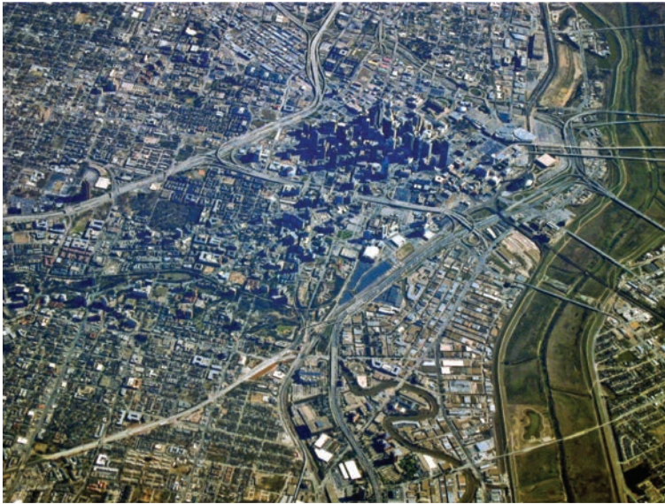
Figure 15.32 An aerial view of Dallas, United States, and the Trinity River parkway. The parkway has levees on either side to protect the city from flooding but the park has been designed as a series of wetlands to accommodate water during heavy rainstorms when the drainage capacity of the river channel is exceeded (Credit: G. Paccaloni; with permission).
