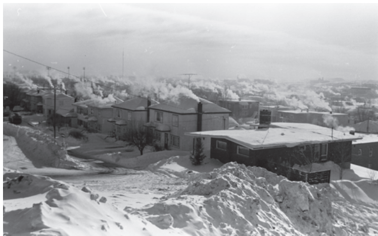
Figure 8.9 Condensation plumes from houses in a northern city (Rouyn, Canada) where natural gas is burnt in furnaces to provide space warming. This illustrates the anthropogenic water vapour injected into the urban atmosphere (Credit: CMHC, used with permission).
