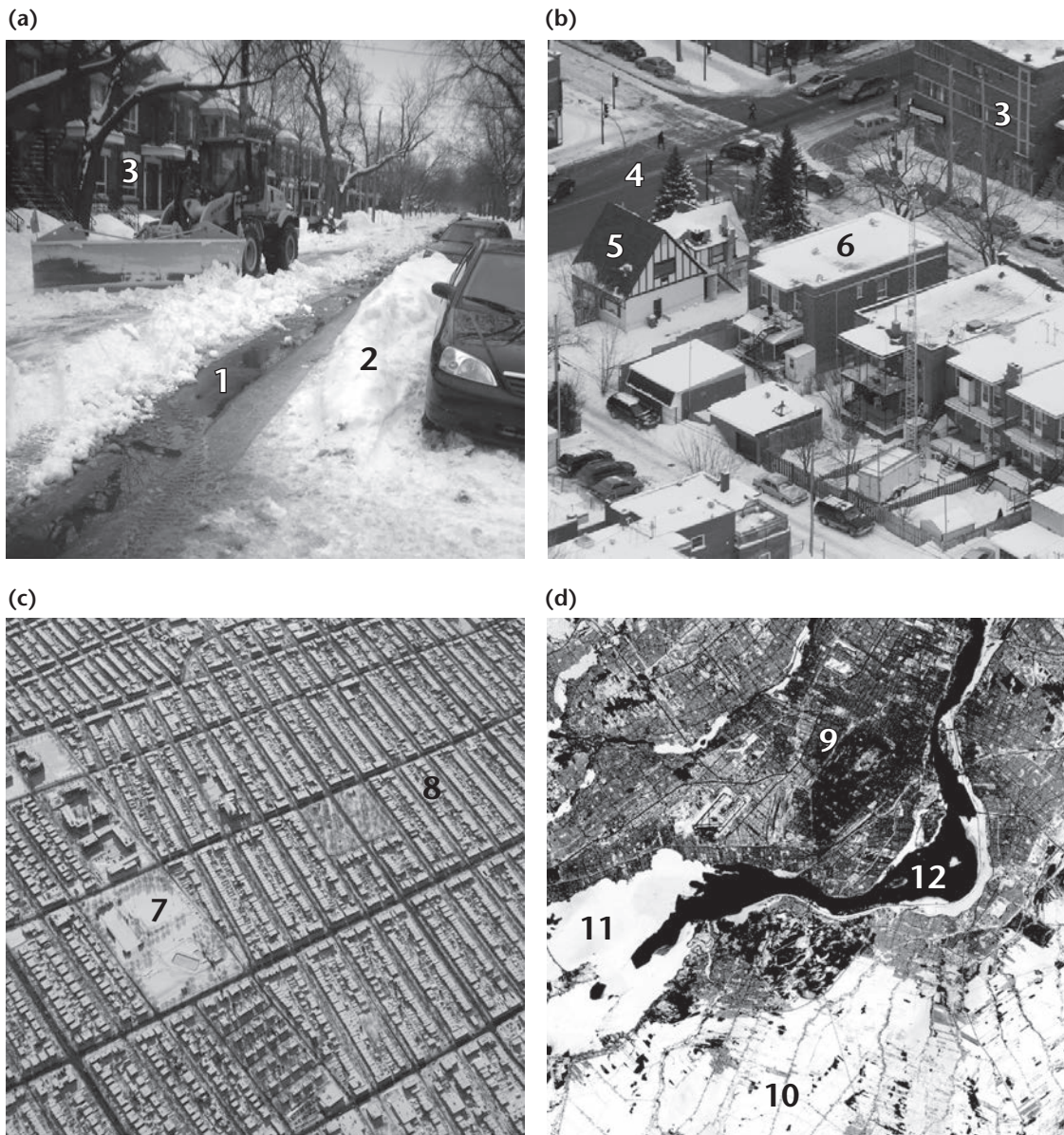
Figure 5.18 Impacts of urban structure and human activity on the darkness (related to the albedo) of Montreal, Canada, when covered in snow at different scales: (a) canyon (Credit: E. Christensen), (b) canyon/urban block (Credit: J. Voogt), (c) neighbourhood (Credit: J. Voogt), and (d) city (Credit: USGS/NASA Landsat Program). Impacts and surfaces: 1 – snow clearance, 2 – soiling/tracking by cars and snow piles, 3 – snow-free walls, 4 – snow removal on main roads, 5 – snow-free pitched roof, 6 – snow pack on flat roof, 7 – undisturbed snow in park, 8 – residential area, 9 – city, 10 – countryside, 11 – snow on river ice, 12 – ice-free river.
