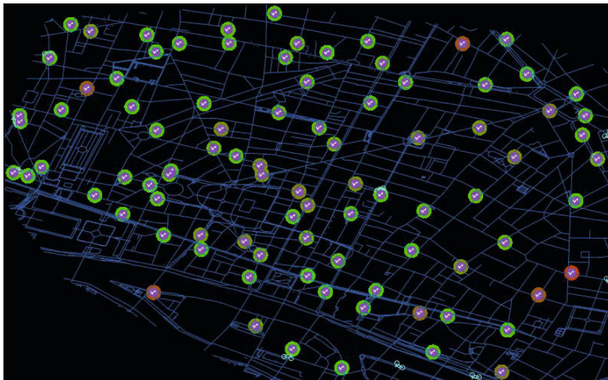
Fig. 2 Example of the graphical output of the model for a particular district (Chatelet). The map shows docking stations, for each the color gradient from green to red gives the current loading factor (green : empty, red : full).
