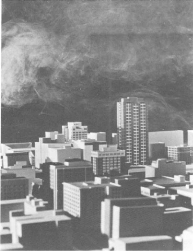
Fig. 1.6 Wind-tunnel model of urban airflow, simulating Denver, Colorado. (Courtesy of Professor J. E. Cermak, State University of Colorado.)
