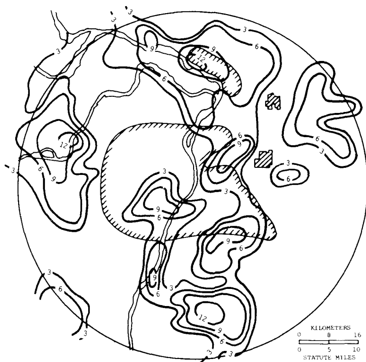
Fig. 8.3 Composite distribution of cloud condensation nuclei at 600 m above mean sea level observed over the St. Louis area during flights 1971–1975. Iso-lines give nuclei numbers of 10^4 \text{ cm}^{-3} (from Semonin, 1978).
