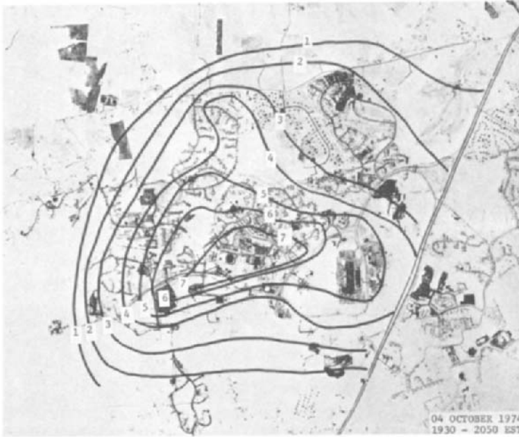
Fig. 5.8 Maximum heat island at Columbia, Maryland, in 1974 when town had grown to 20,000 inhabitants. (From Landsberg, 1975.)
