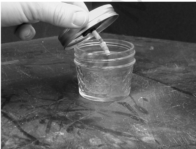
Figure 10.15 (a) Schematic drawing and (b) photograph of typical laboratory set up for measuring total soil suction using thermocouple psychrometer.
