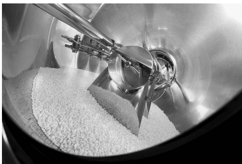
FIGURE 3.4 Film-coating process in the Pellegrini pan with immersion swords. (Courtesy of IMS S.p.A.)
