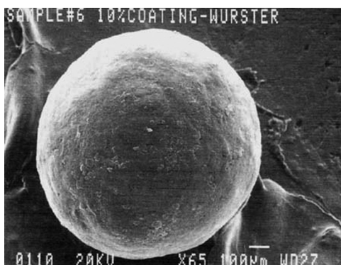
FIGURE 2.41 Surface view of PPA-HCl seed coated by Wurster method. PPA, phenylpropanolamine.
