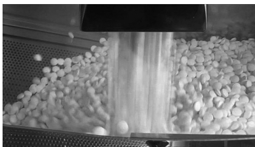
FIGURE 3.11 Tablet feed into the first chamber.
