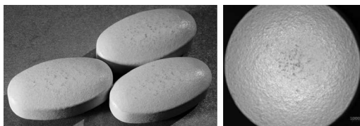
FIGURE 5.36 (See color insert.) Examples of surface scuffing of film-coated tablets.
