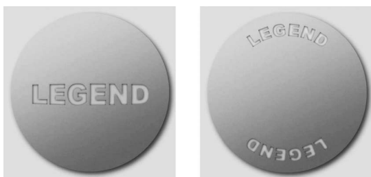
FIGURE 5.17 Schematic diagram illustrating options for tablet logo placement.
