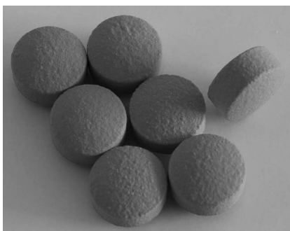
FIGURE 5.28 (See color insert.) Example of unacceptably rough film-coated tablets.
