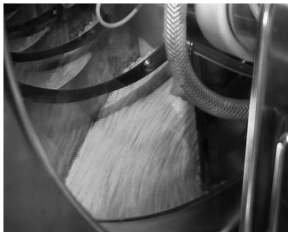
FIGURE 3.12 Tablet inter-chamber transfer.
