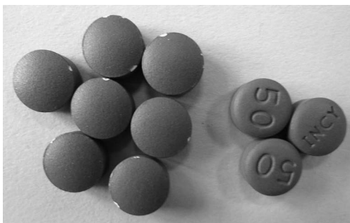
FIGURE 5.13 (See color insert.) Example of how changing from standard concave punches to compound radius punches can eliminate tablet edge chipping.
