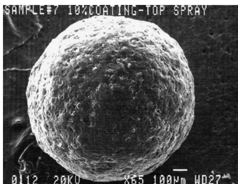
FIGURE 2.40 Surface view of PPA-HCl seed coated by top spray (granulating) method. PPA, phenylpropanolamine.
