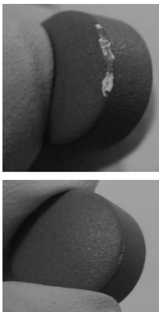
FIGURE 5.9 Example of film-coated tablet edge chipping. (© 2015 AstraZeneca, all rights reserved. Image reproduced with permission of AstraZeneca; image is copyright of AstraZeneca and may not be reproduced without written permission.)
