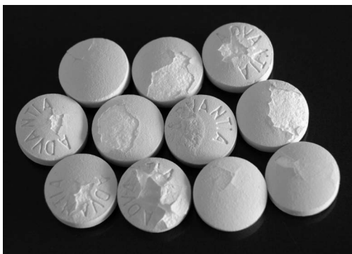
FIGURE 5.20 (See color insert.) Example of film peeling and flaking.
