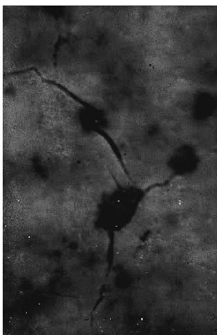
FIGURE 5.27 Example of cracking initiated by poorly dispersed pigments.
