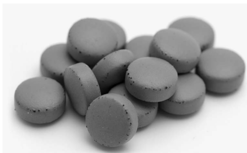
FIGURE 5.33 Tablet discoloration caused by bleed-through of ingredients from tablet core.
