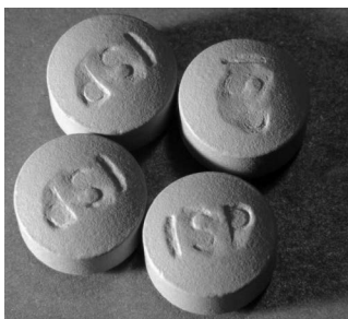
FIGURE 5.16 Photograph illustrating how the presence of a logo in the center of the tablet can have a negative impact on tablet surface erosion.
