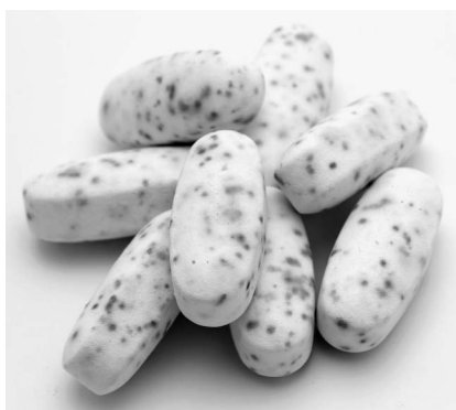
FIGURE 5.32 (See color insert.) Tablet discoloration caused by interaction of ingredients in the tablet core.
