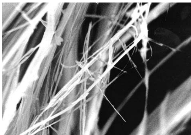
Figure 2.1 Chrysotile asbestos fibers under microscopic magnification. (Courtesy of Hibbs, L., McTurk, G., and Patrick, G., MRC Toxicology Unit, Leicester, U.K.)
