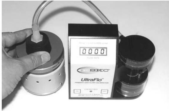
Figure 9.11 Calibration of a total mold spore/particle sample device.
