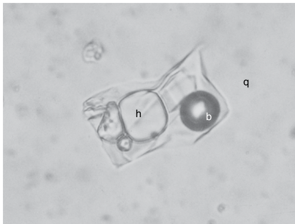
Figure 4.6.1 Thin section view of a fluid inclusion (about 30\mu\text{m} across) from a quartz vein in the Dartmoor Granite, Devon, England. h=halite crystal, b=gas bubble, q=host quartz crystal. The gas bubble boundary appears more prominent (in optical terms, it has higher relief ) because of the high contrast in refractive index between the gas and the surrounding liquid. (Source: Photo courtesy of Dr D. Alderton.)
