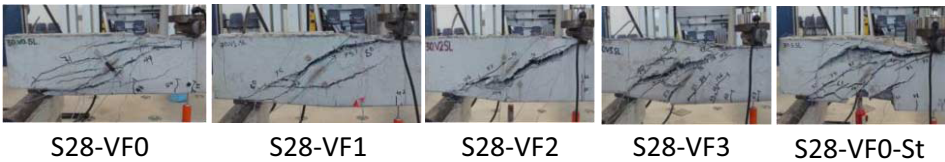
Figure 3. Failure modes of the slender specimens of group (A)
