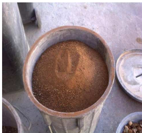
Figure 1. Demolished waste sand
