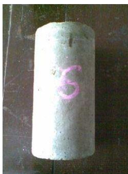
Figure 8. Concrete surface after five cycle immersion in sulphate solution
