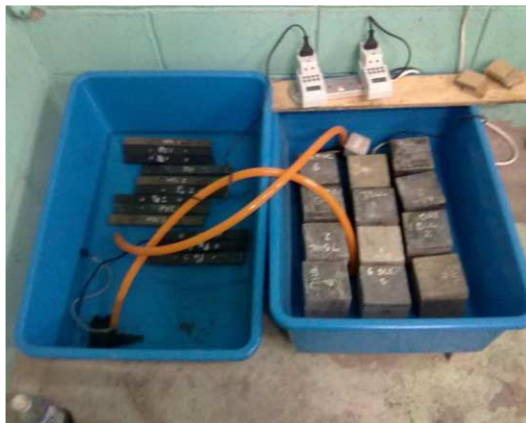
Figure 1. Specimen in sulphate solution with alternate wet and dry cycle arrangement.
