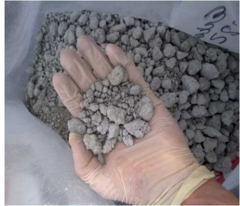
Figure 4. Returned Ready-Mix concrete (dry)
