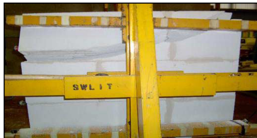
Figure 1. Typical failure of a low density aircrete thin layer (mortar) walette in the B direction showing predominantly material failure
