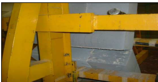
Figure 2. Typical failure of a low density aircrete thin layer wallette (after 1 day curing) in the B direction showing failure occurring along the bed joint.
