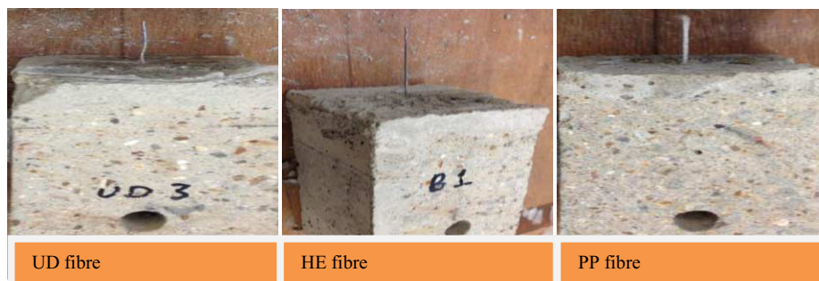
Figure 4. Pull-out failure of fibres
