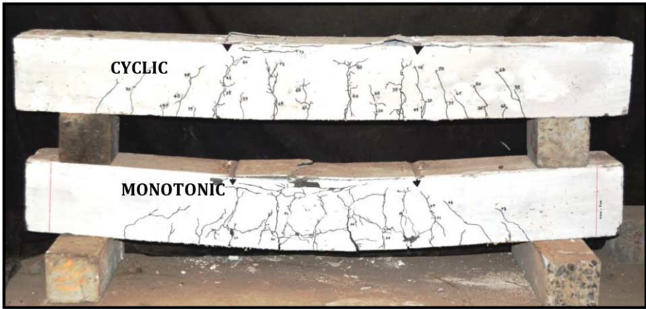
Figure 6. Crack pattern in SFRSCRC beams under monotonic and cyclic loading
