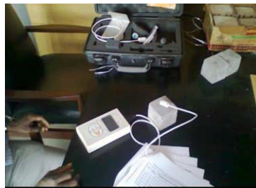
Figure 3. KD 2 Pro-Thermal analyzer during measuring of mortar properties
