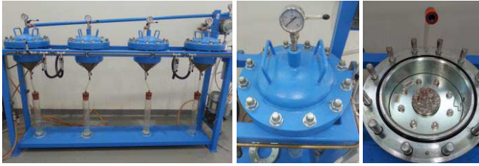
Figure 1. Water permeability test
