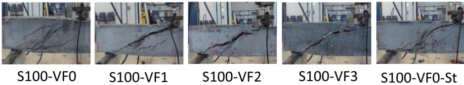
Figure 5. Failure modes of slender specimens of group (B)
