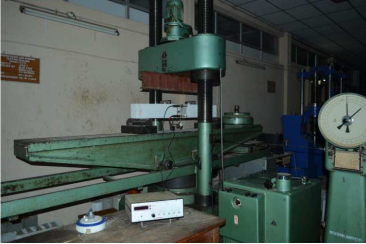
Figure 3. Test setup for monotonic and cyclic loading test on beams
