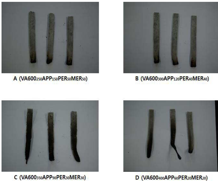
Figure 3. Combustion sample of flame retardant test by UL 94
