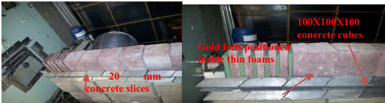
Figure 4. Experimental set up with foil
