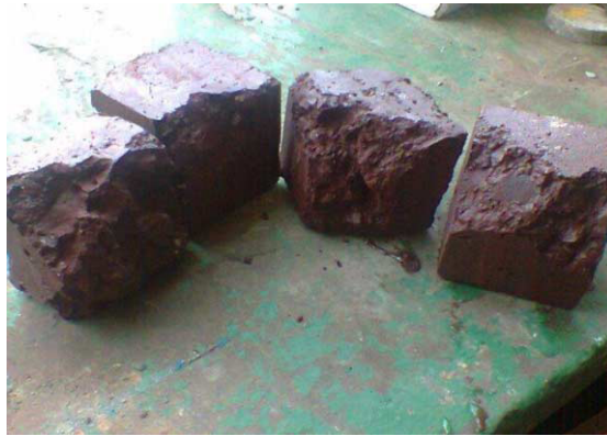
Figure 1. Disintegrated cubes after being placed under water following the use of colemanite
