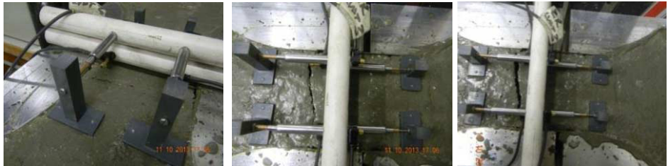
Figure 5. LVDT displacement measurement setup over gauge length.
