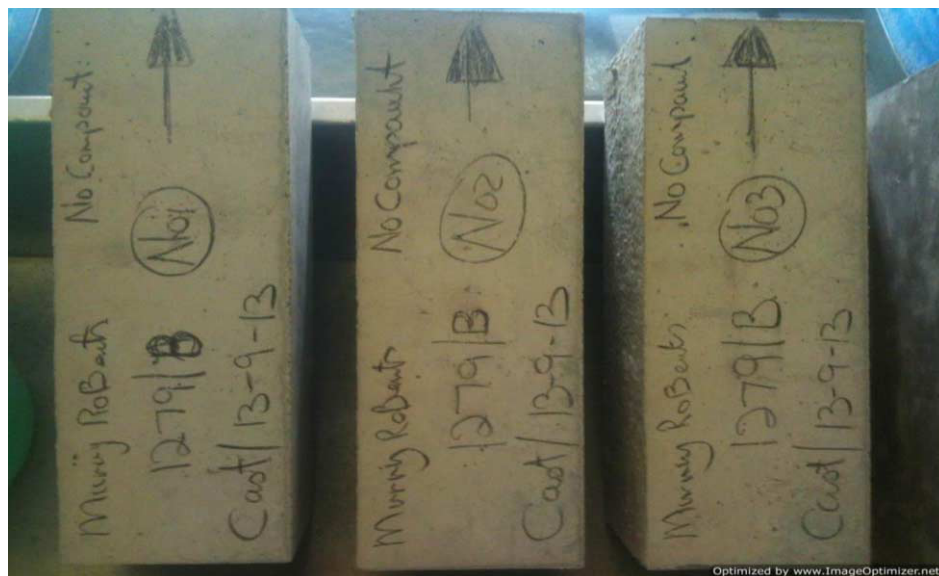
Photo 3. Alkali-activated concrete test specimen from site tested for shrinkage.
