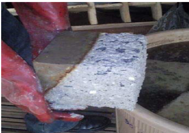
Figure 3. Typical leaching of \text{Ca}(\text{OH})_2 from concrete cubes in the \text{H}_2\text{SO}_4 solutions at 90-day curing age
