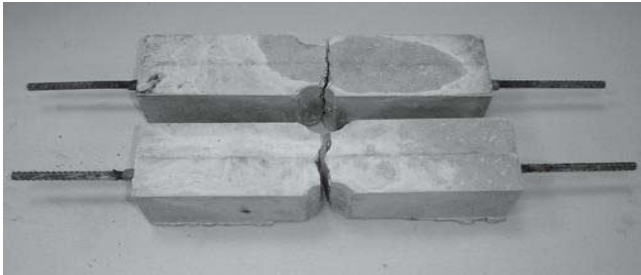
Figure 7. Typical direct tensile failure
