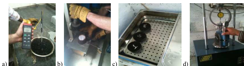
Figure 3. Marshall specimen preparation: a) Material mix after heating, b) Specimen compaction, c) Specimens in water bath and d) Marshall test machine.
