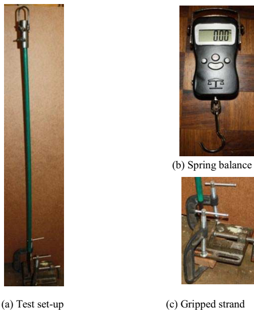
Figure 2. Friction test apparatus
