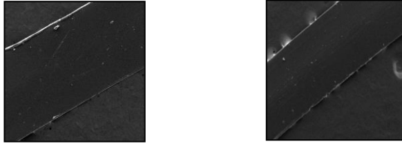
Figure 1. SEM micrograph of sample 5644 both pre and post artificial UVA exposure
