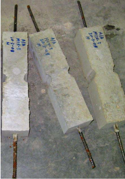
Figure 5. Shape of direct tension specimen
