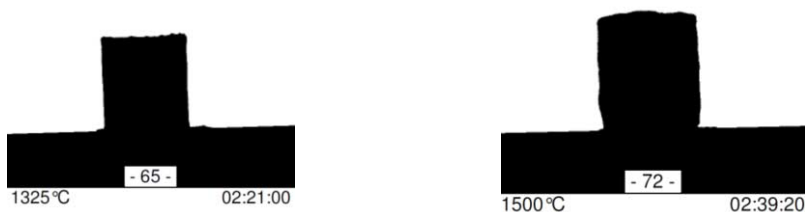
Figure 4. Sample BFA2 at maximum sintering and maximum swelling at the end of the test
