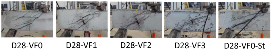
Figure 4. Failure modes of the deep specimens of group (A)
