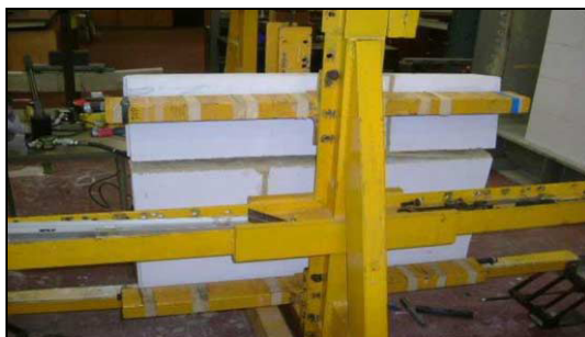
Figure 3. Typical failure of a low density aircrete designation iii wallette in the B direction showing failure occurring along the bed joint.
