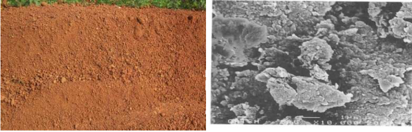
Figure 1. (a) Lateritic soil/gravel (b) Microstructure of lateritic soil
