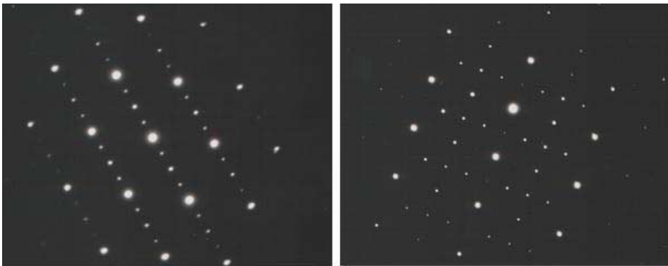
Figure 4. Electron diffraction patterns taken from CuZnAl and CuAlMn alloy samples
