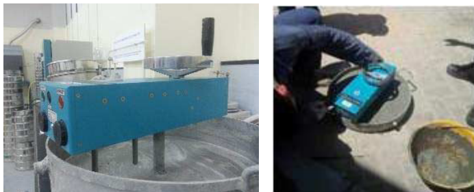
Figure 1. Illustration of the concrete rheometer used: (a) rheometer assembled, (b) rheometer during testing rheology of fresh concrete
