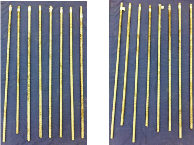
Figure 5. Top reinforcing steel recovered from Panels 3A and 5A with 20 \text{ l/m}^3 of DCI and CNI respectively
