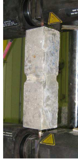
Figure 6. Direct tension test in progress
