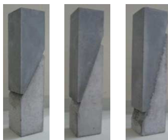
Figure 2. Real illustration of the slant shear specimens
