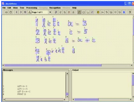
Fig. 3. Screenshot of JMATH, the editor and training program for formula recognition developed by E. Tapia, coupled to the BASIC interpreter.
