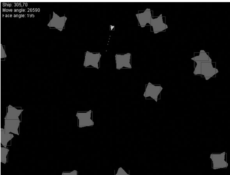
Figure 3.3 Bounding rectangles are used to detect when collisions occur.
