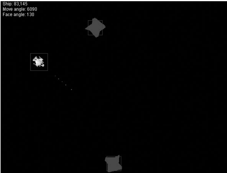
Figure 11.2 The bounding rectangles are used for collision testing.
