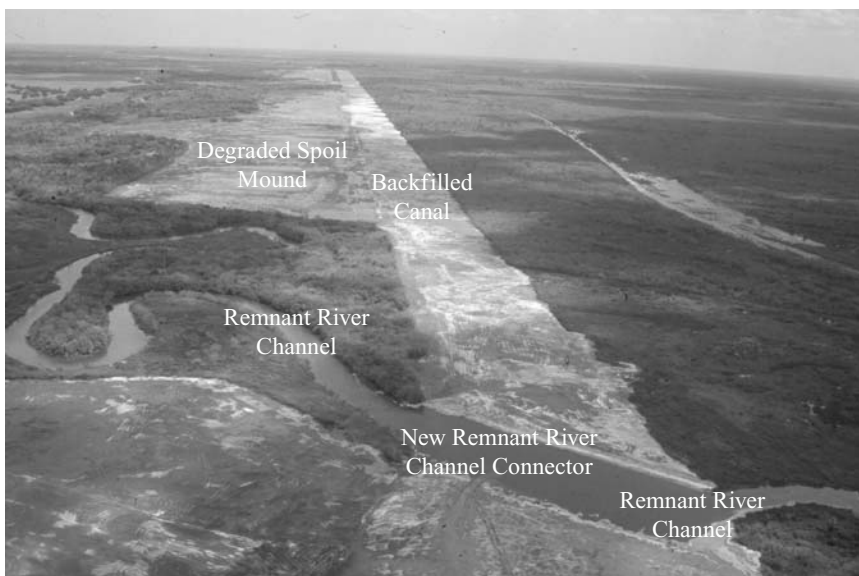
Figure 6-10. Recently (June 1999–February 2001) backfilled flood control canal, degraded spoil mound, and reconnected remnant Kissimmee River channel. The new remnant river channel connector spans a portion of the flood control canal that was backfilled to a depth of 3 to 4 m, which is consistent with the bottom elevation of the reconnected remnant channels. (Photograph by Paul Whalen, South Florida Water Management District; used by permission.)
