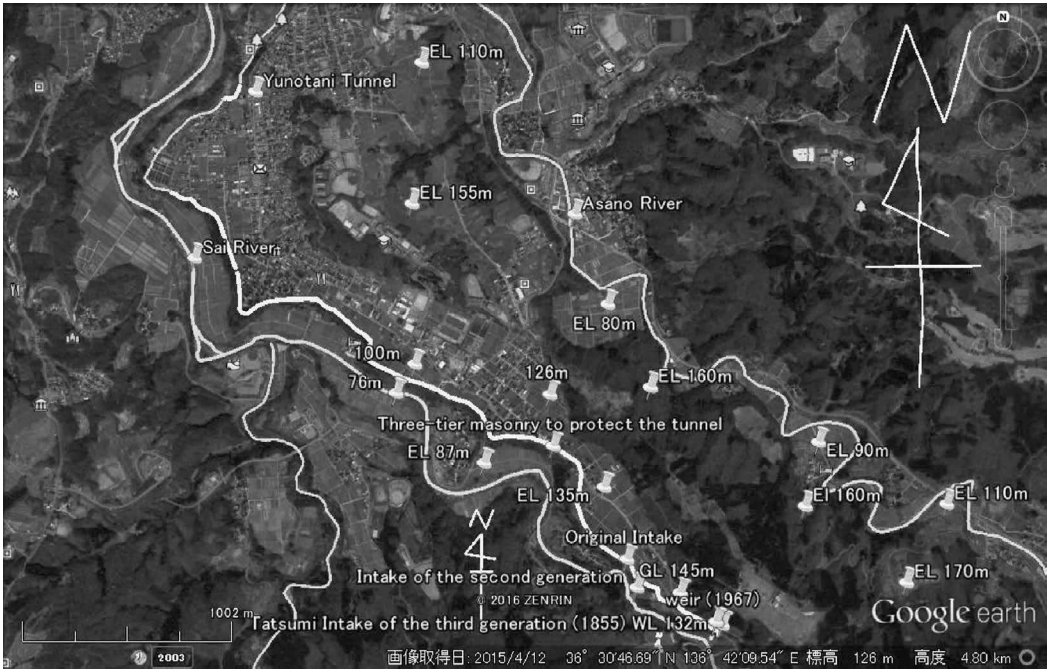
FIGURE 21.4 Alignment of the tunnel on Google Earth shows close location to the scarp of the Otarui Terrace. (From HP/Google, Tatsumi Aqueduct, 2015a. With Permission.)
