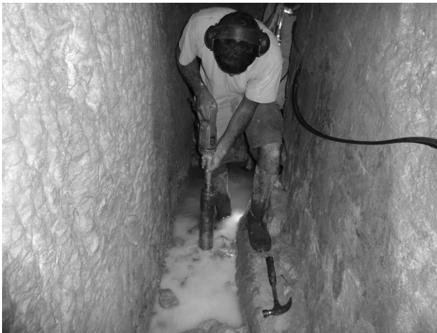
FIGURE 10.14 Joweizeh spring. Drilling a core at the bottom of the spring tunnel. (Photography by Yechezkel.)
