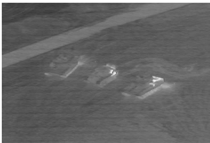
Figure 7.16 Close-up image taken from a helicopter with a TICM-II camera (8–12 \mu\text{m} ).
