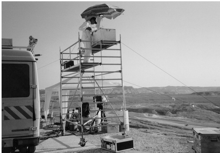
Figure 7.70 Measurement setup with SCORPIO (Section 5.2) on top of scaffold and the DuDa imager (Section 6.4) to the left under a party tent.
