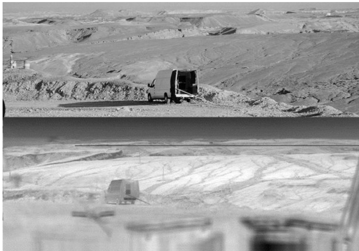
Figure 7.71 Visual and infrared (DuDa 8–12 \mu\text{m} ) image of the calibration setup. Blackbodies are placed inside the van to shield from solar irradiance.
