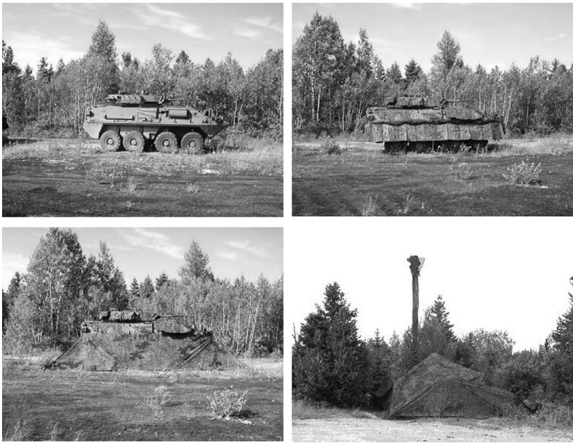
Figure 8.19 MCS applied to the Canadian COYOTE. Original (top left), permanent measures (top right), short halt (bottom left), and longer halt (bottom right). (Courtesy Canadian Forces.)
