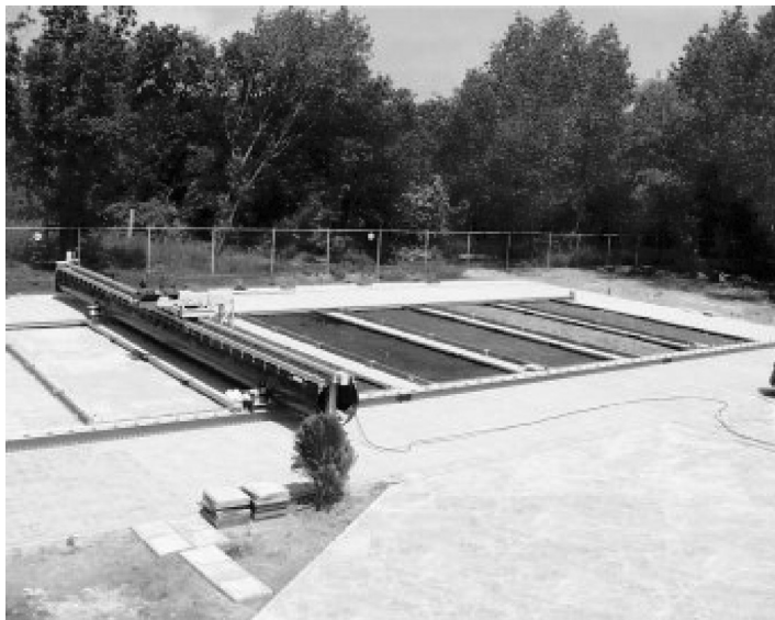
Figure 7.18 Test bed to measure multispectral signatures of surface and buried land mines.
