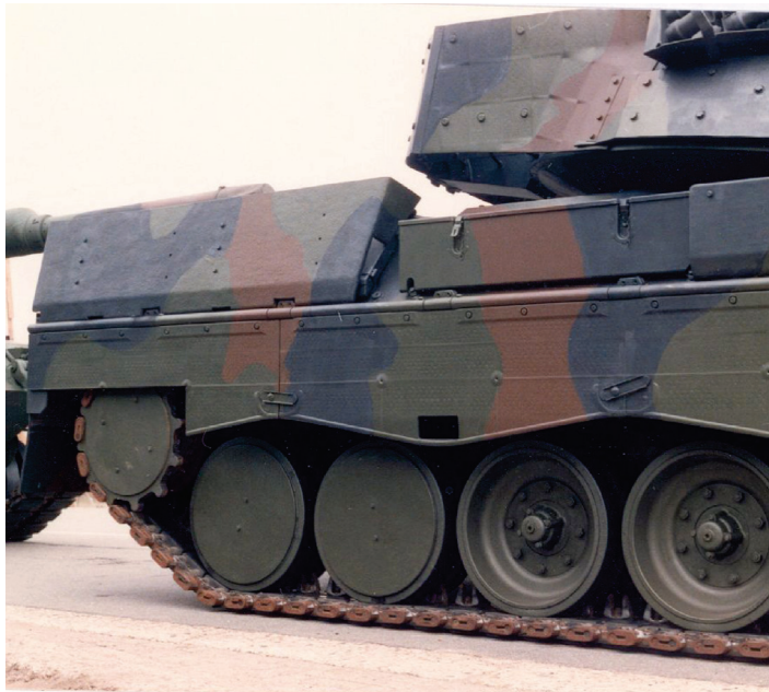
Figure 8.5 Target modifications to reduce the visible and infrared signature.
