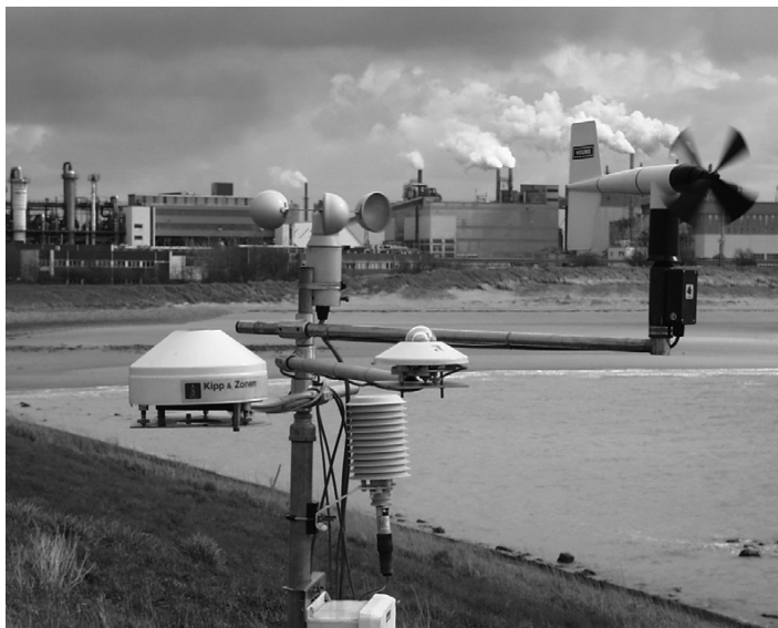
Figure 5.1 Portable meteorological station set up in a coastal environment.
