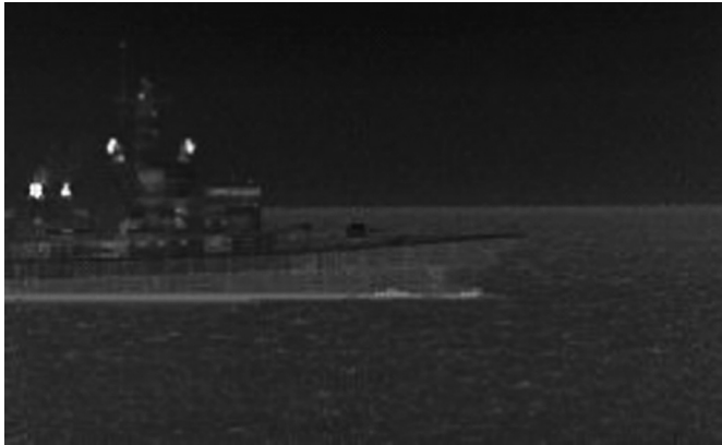
Figure 3.8 Thermal image of a ship at sea, showing various hot sources.
