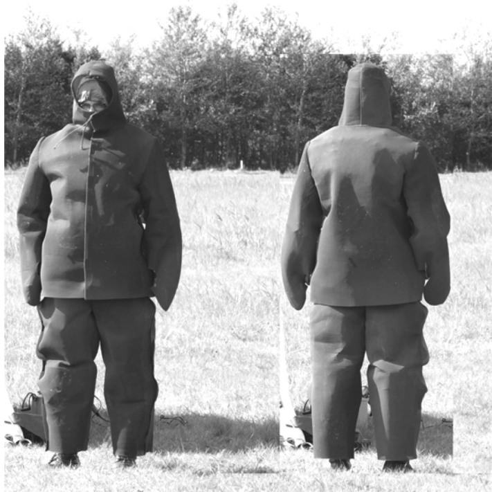
Figure 8.23 Suit with reduced heat conduction, created by a 10-cm air space.
