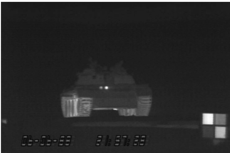
Figure 6.17 T62 placed on the turntable (8–12 \mu\text{m} ).
