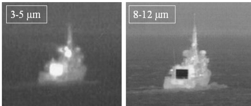
Figure 8.7 IR signature of hangar door on the rear deck of a frigate.
