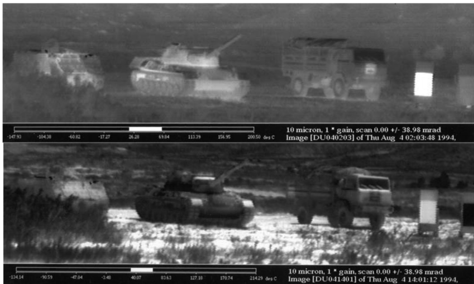
Figure 7.6 CHAR-II DuDa 8–12 \mu\text{m} images of targets in position 1 (SE) during early night (top) and early afternoon (bottom).
