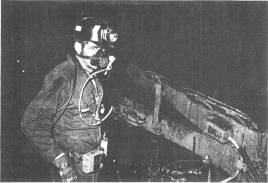
Figure 26.3 An underground coal miner wearing two personal air samplers during a respirator test.
