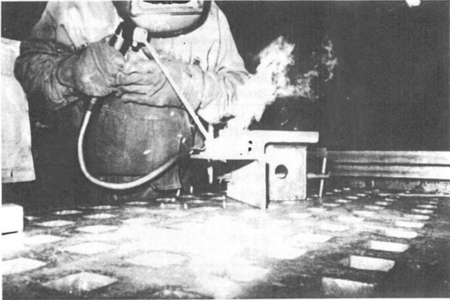
Figure 10.2 A welder striking an arc with a shielded electrode. The welder is wearing a helmet with a welding plate and appropriate protective clothing.
