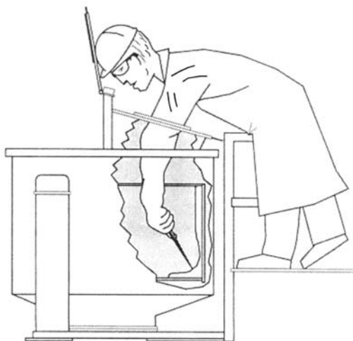
Figure 16.13 Glove-port system on centrifuge. Operator is wearing chemical splash goggles.
