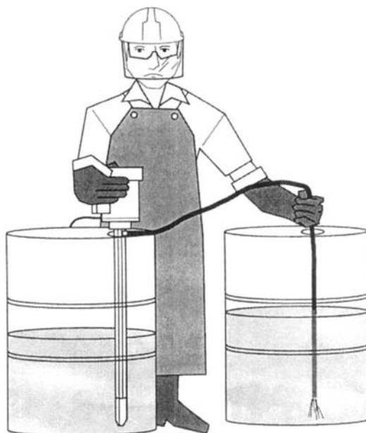
Figure 16.5 A drum pump. Operator is wearing chemical splash goggles and faceshield. Containers are electrically bonded.
