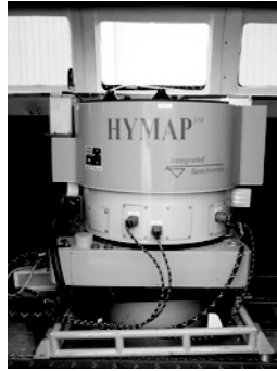
Figure 14.10 View of HyMap™ hyperspectral scanner ( http://www.hyvista.com/hymap.html ).
