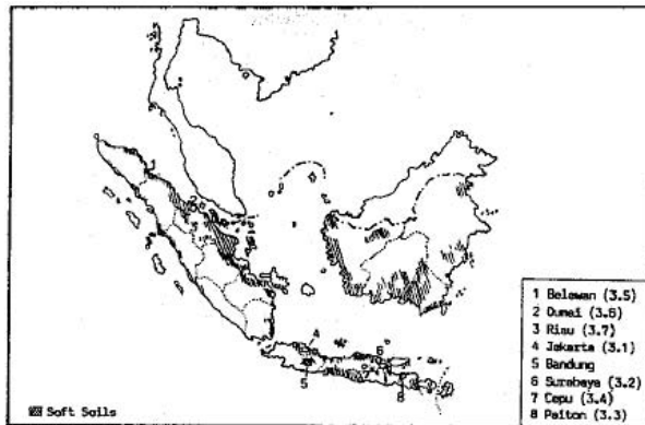
Figure 30.11 Location of major area of the soft soil in Indonesia.
