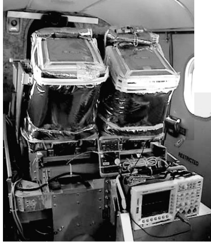
Figure 14.8 View of AVIRIS hyperspectral sensor inside the Twin-Otter aircraft ( http://aviris.jpl.nasa.gov ).
