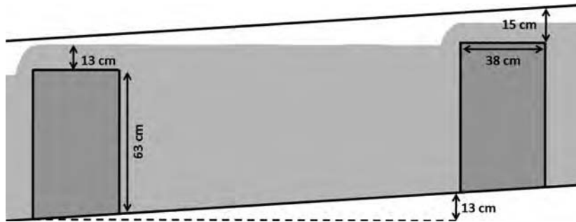
Figure 13.22 Schematic representation of the water flow in the channel at the centre of Perge's main street
