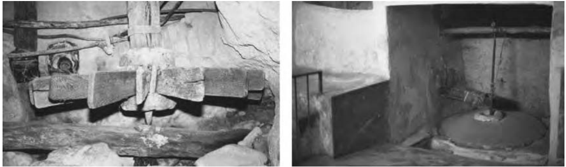
Figure 5.31 Water mills: paddles in Taft in the province of Yazd (left) and upper millstone in Kashan (right)
