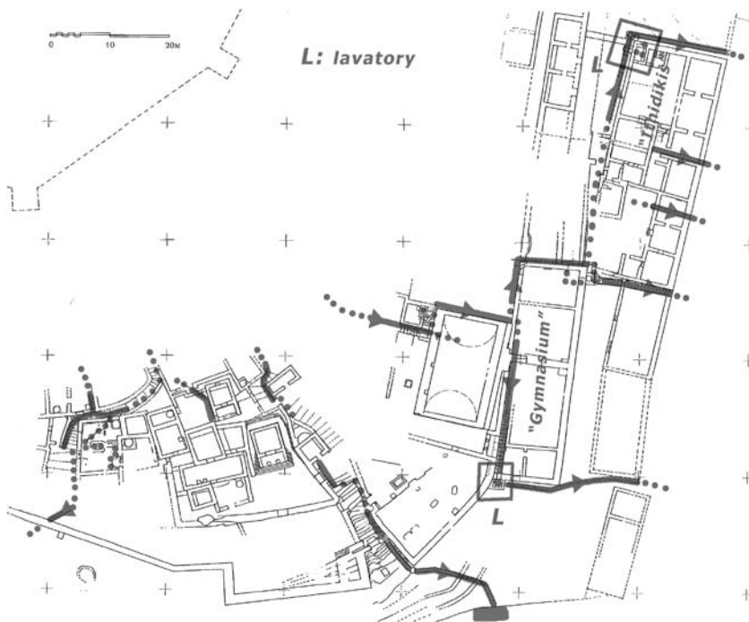
Figure 6.15 Minoa on Amorgos. Drainage pipe work facilitating also reuse of water (with permission of G. Antoniou).
