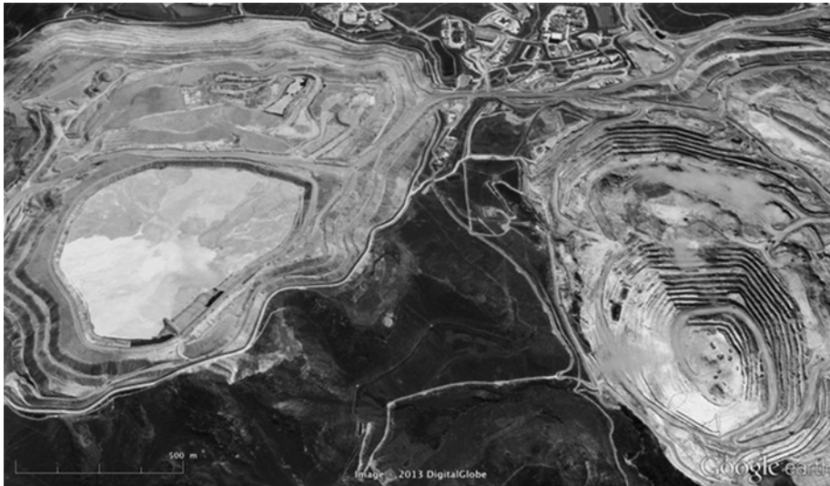
Figure 5.24 Satellite view over a section of the Yanacocha open pit gold mining site, showing a leaching pond on the left, and an open pit on the right. The image encompasses an area of about 2.400 m × 1.400 m. The total area of the Yanacocha mining site surpasses the urban area of the nearby city of Cajamarca. Source of satellite view: Google earth.
