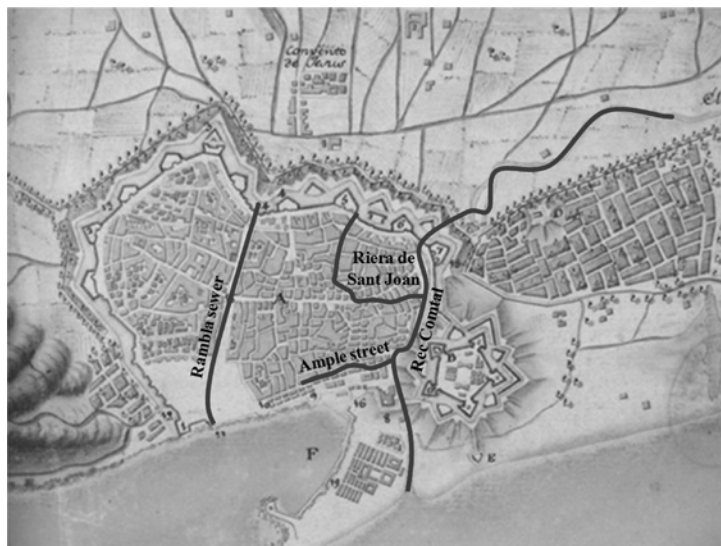
Figure 19.4 Scheme of the main sewers existing in Barcelona at the end of the 18th century (Barcelona City council, 1986).
