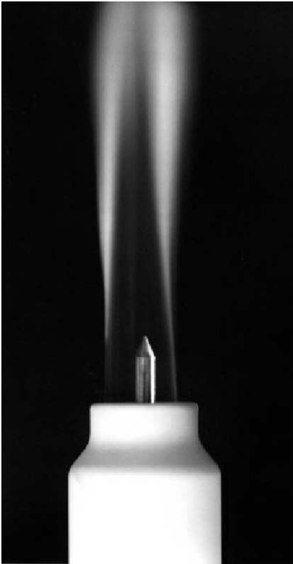
6.12 Demonstration of laminar flow by use of gas lens. Courtesy of TWI Ltd.
