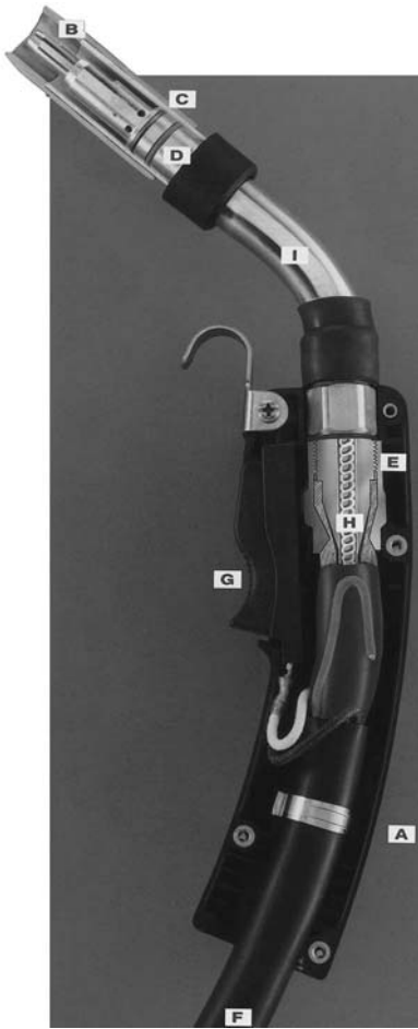
7.10 Exploded view of a typical MIG torch: A ergonomically shaped handle; B contact tip, C gas shroud, D gas diffuser, E power cable connector, F umbilical containing gas hose, power cable and control cable, G power switch, H replaceable liner, I adjustable nozzle. Courtesy of Bernard Welding Equipment Company.
