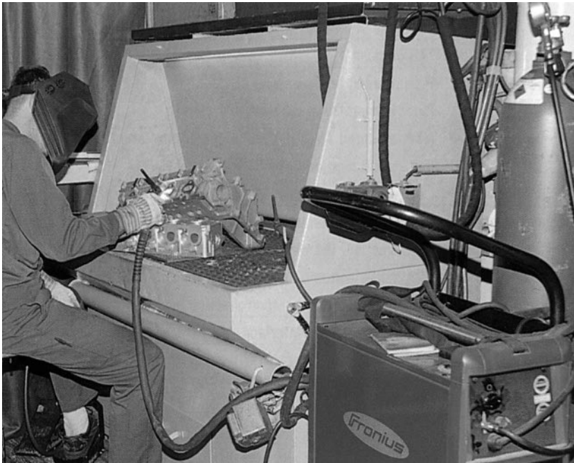
6.2 Manual DC-ve TIG welding repair of aluminium castings using helium shielding gas. Courtesy of TPS-Fronius Ltd.
