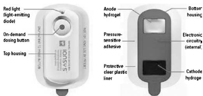
Figure 20.1: Fentanyl iontophoretic transdermal system: Front and back view.
