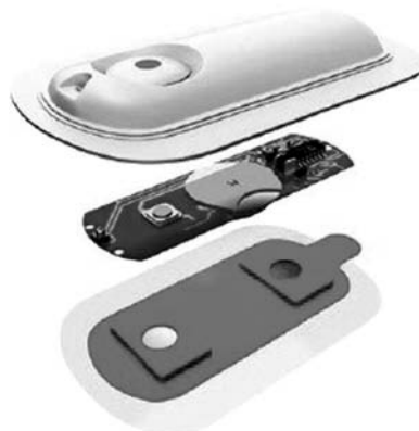
Figure 20.2: Fentanyl iontophoretic transdermal system: Electronic and drug components.
