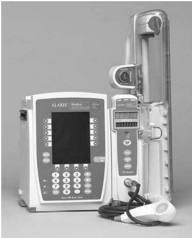
Figure 19.9: The Alaris System is the forefront of PCA safety technology. Its platform is capable of integrating PCA, \text{SPO}_2 , capnography ( \text{ETCO}_2 ), and bar coding for all infusions, with wireless connectivity to transmit pertinent data to existing clinical information systems and electronic patient records. (Figure courtesy of Alaris Medical Systems, Inc, subsidiary of Cardinal Health, Inc, San Diego, CA.)
