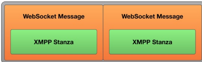
Figure 4-6. No stanza-to-message alignment (WebSocket to TCP proxy)
