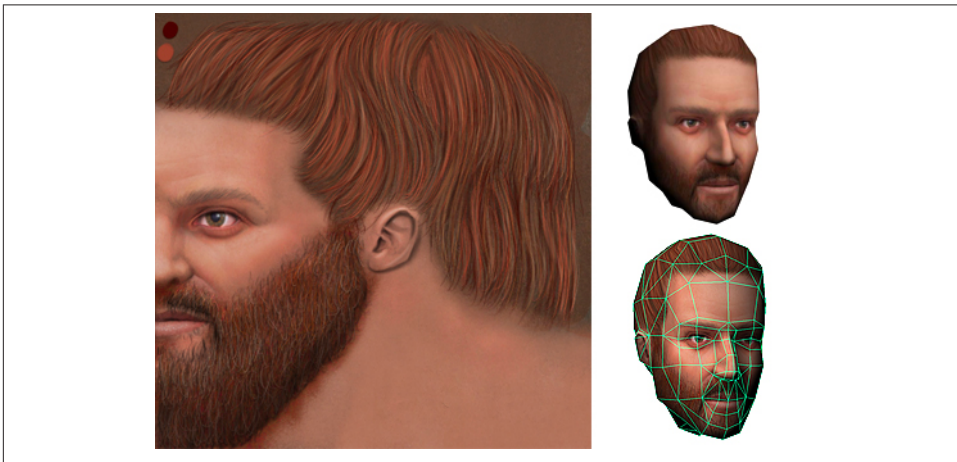
Figure 8-2. Texture mapping: a 2D image is wrapped and reflected onto the surface of a 3D object (image courtesy Simon Wottge )
