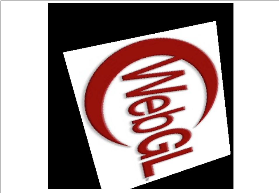
Figure 2-4. gl.NEAREST filtering: textures are pixelated in close-up objects
