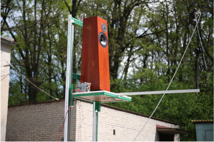
Fig. 6.37 The open-air the loudspeaker system measurement
