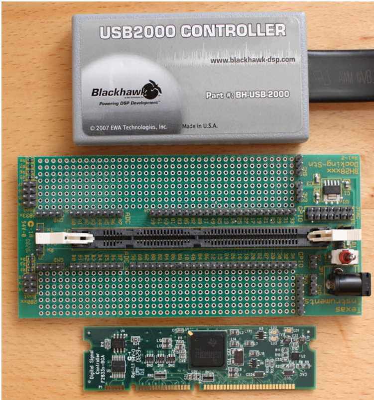
Fig. 3.82 System for developing software and hardware: F28335 control card, CC28xxx docking station and USB2000 Controller
