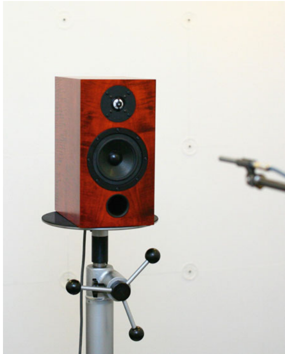
Fig. 6.39 The digital active loudspeaker system under the tests
