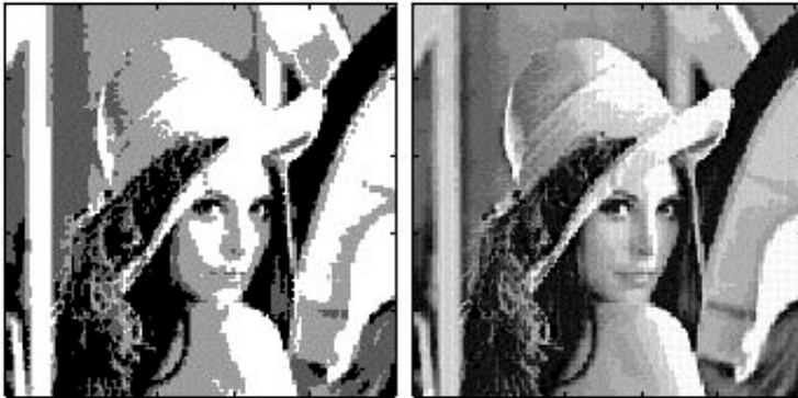
Figure 12.38 – LBG compression: ( m = 4, b = 2 ) on the left, ( m = 4, b = 4 ) on the right
