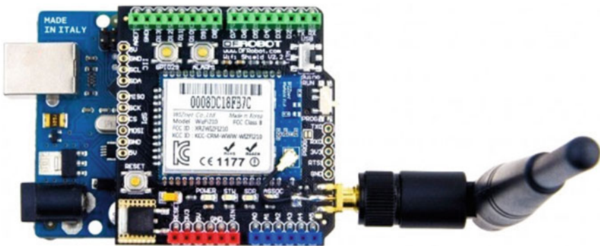
Fig. 5.22 A diagram of the layout of the Wi-Fi module v2.2 and UNO R3
