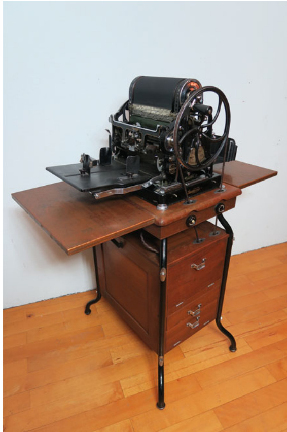
Fig. 8 The Gestetner mimeograph, before it was redesigned by Raymond Loewy. Photo by Carsten Sadowski. URL: http://www.ebay.de/itm/Rare-duplicator-copy-machine-by-D-Gestetner-Tottenham-London-ca-1927-Model-15-/251955002475?nma=true&si=NNKp%252BhPnvzOiYsZyMB5kOEwaSYk%253D&orig_cvip=true&rt=nc&_trksid=p2047675.12557
