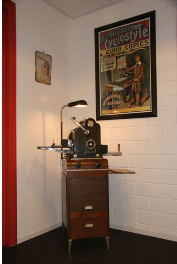
Fig. 9 The Gestetner mimeograph as redesigned by Raymond Loewy. Photo by Erwin Blok, courtesy of stencilroloFlick/Flickr.com. URL: https://flic.kr/p/5NQPUK
