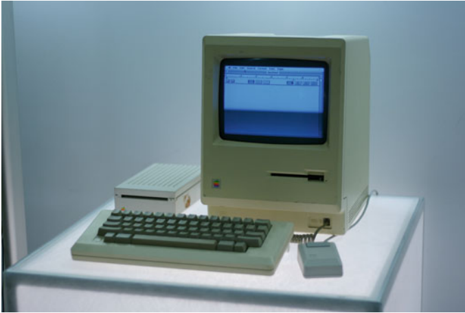
Fig. 3 Original Macintosh 128 k, made in 1984. Note the absence of cursor keys on the keyboard. Photo by Marcin Wichary. URL: https://flic.kr/p/4jA1sX
