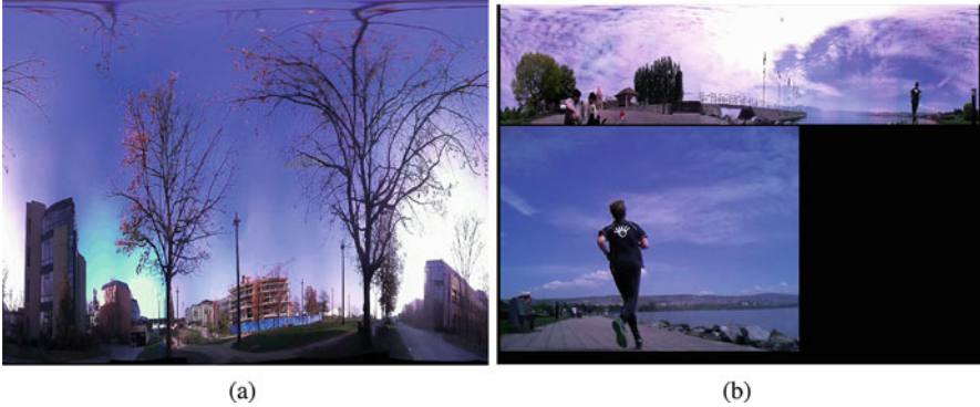
Fig. 6.10 (a) Omnidirectional snapshot of resolution 1024 \times 768 for the linear interpolation technique. (b) Omnidirectional snapshot of resolution 1024 \times 256 for the nearest neighbor interpolation technique plus VGA ( 640 \times 480 ) display of a single selected camera
