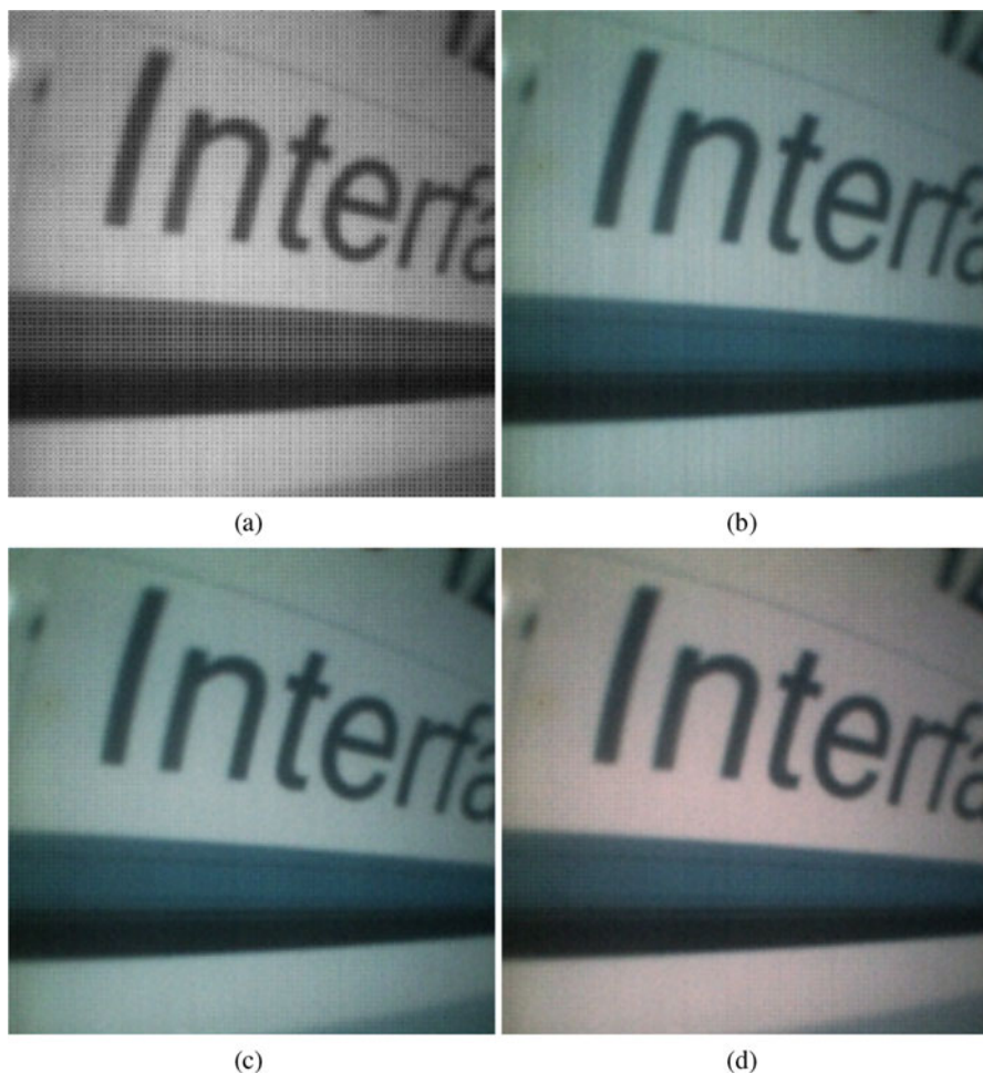
Fig. 7.11 An example of the effect of Raw Image Processing on the final image. (a) The raw input image shown in grayscale, (b) demosaiced image, (c) denoised and demosaiced image, and (d) denoised, white balanced, and demosaiced image
