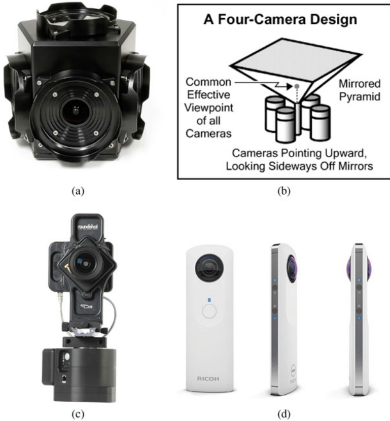
Fig. 2.5 Commercially available panoramic cameras: (a) Pointgrey’s Ladybug5, (b) Working principle of FullView, (c) Seitz Roundshot D3, and (d) Ricoh THETA
