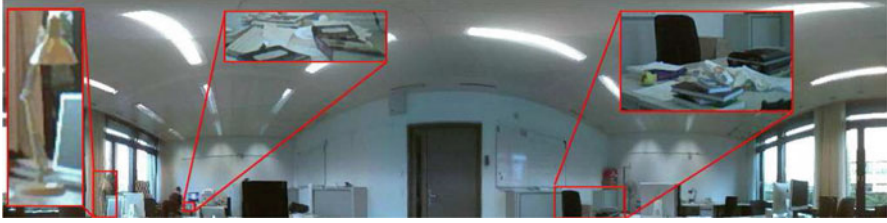
Fig. 3.8 Detailed image parts obtained using Gaussian blending with the grid refinement: a lamp magnified 8\times , the books magnified 32\times , a desk magnified 8\times
