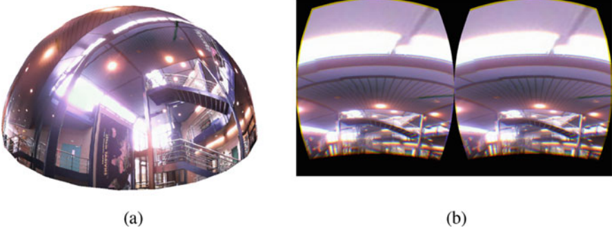
Fig. 6.11 (a) The textured OpenGL hemisphere showing a captured image, viewed from the side. (b) The client application generating the left and right eye view for the head-mounted display
