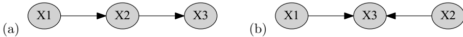
Figure 3.2.3: Directed graphs representing (a) X_1 \perp X_3 \mid X_2 and (b) X_1 \perp X_2 .
