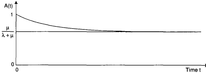
Fig. 9.5 The availability A(t) of a item in Example 9.5, with failure rate \lambda and repair rate \mu .
