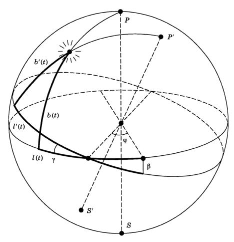
Figure 114. Geometrical representation of systematic errors in terms of spherical coordinates
