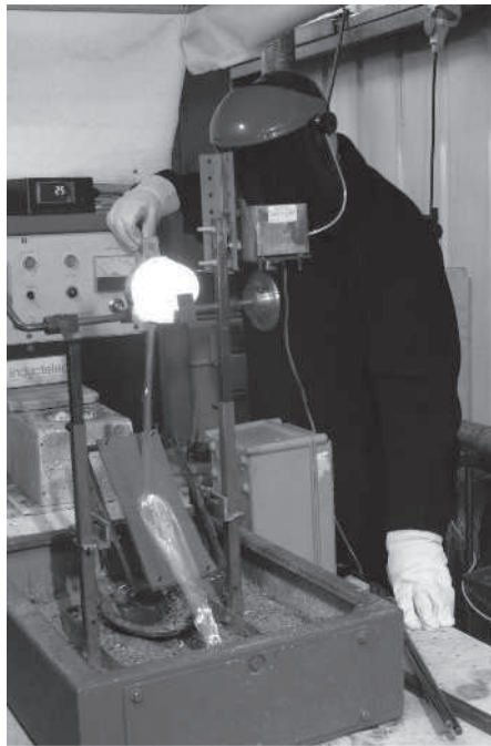
Figure 3.7 The hot metal splash test, BS EN ISO 9185:2007 (replaces BS EN 373:1993). Reproduced with permission from BTTG Fire Testing Laboratory, Altrincham, UK
