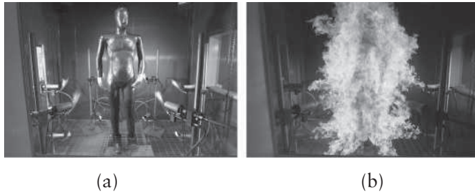
Figure 3.9 Images of the BTTG Ltd., manikin RALPH [68] as (a) the undressed torso and (b) as a manikin under test. Reproduced with permission from BTTG Fire Testing Laboratory, Altrincham, UK
