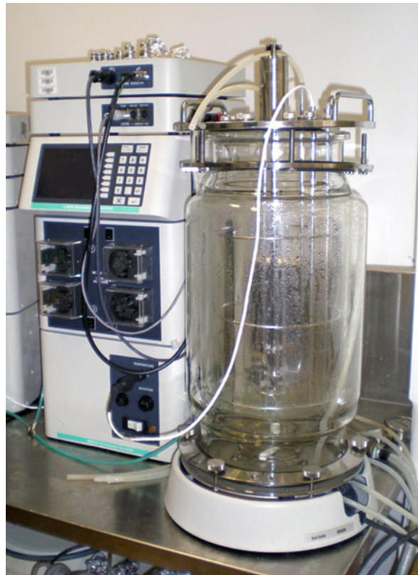
Fig. 2 Fermentation setup for controlled and submerged cultivation of microorganisms such as filamentous fungi, with a capacity of up to 10 L working volume. The picture demonstrates the fermenter control panels on the left with the glass vessel for cultivation on the right
