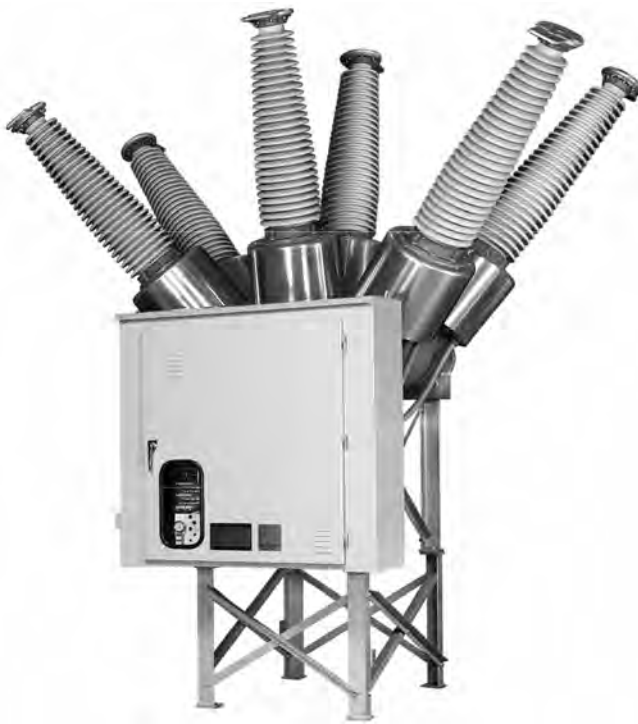
Figure 17.1 Definite purpose, 120 kV, three-phase, 40 kA dead tank SF 6 circuit breaker. (Courtesy of Mitsubishi Electric Products Inc., Warrendale, PA.)
