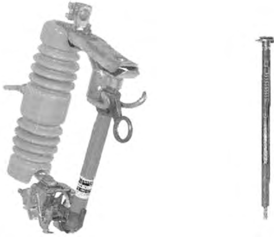
Figure 16.3 View of the cutout for an expulsion type of fuse and a fuse link. (Courtesy of S&C Electric Company, Chicago.)
