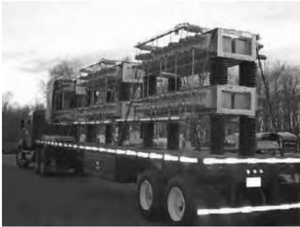
Figure 7.12 A mobile capacitor bank. (Courtesy of Gilbert Electrical Systems and Products, Beckley, WV.)
