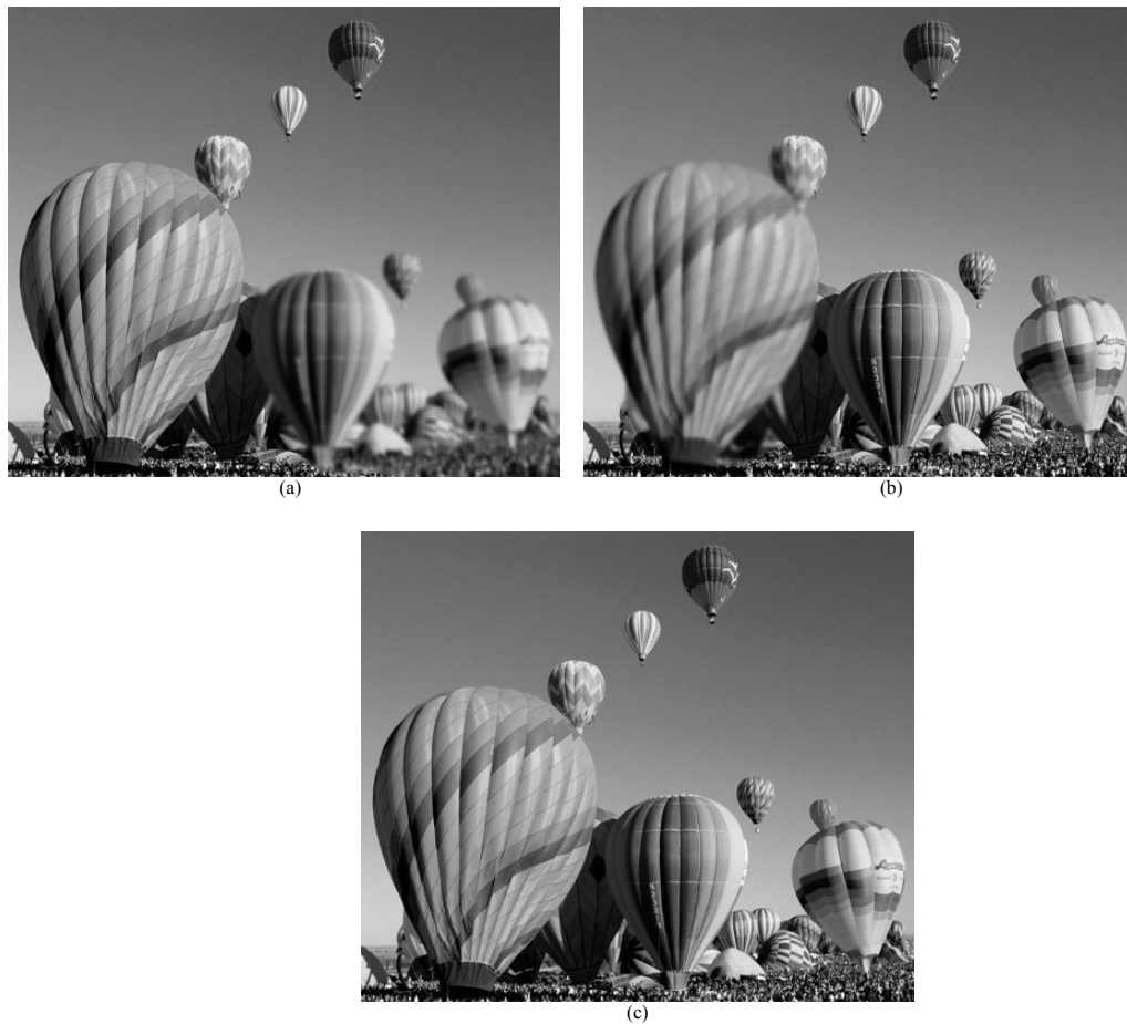
FIG. 2 (a) IMAGE WITH RIGHT HALF IN BLUR (b) IMAGE WITH LEFT HALF IN BLUR (c) FUSED IMAGE USING PROPOSED SCHEME.
