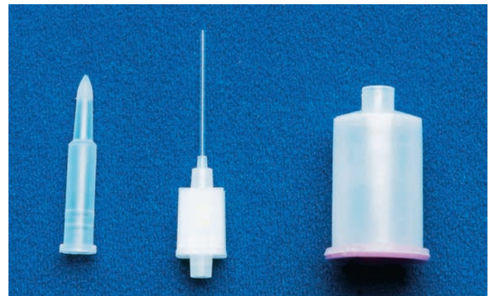
■ FIGURE 11 Unopette system (from left to right): pipet shield, pipet, and reservoir.
