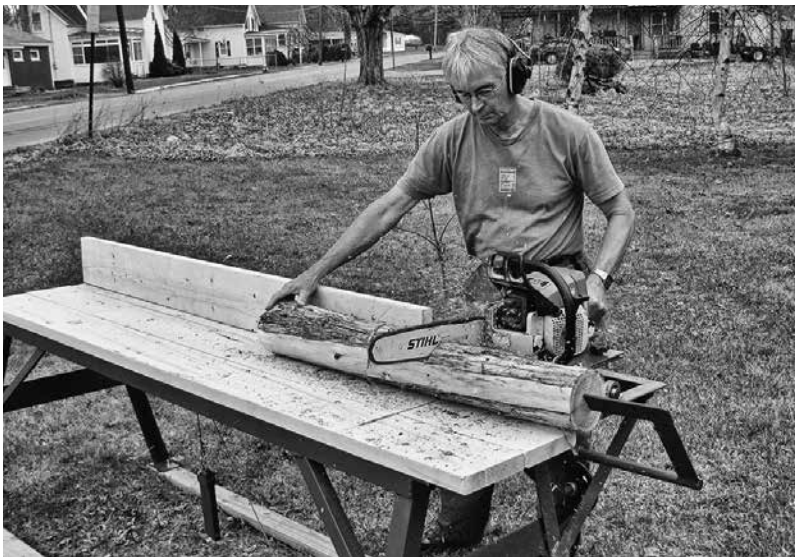
12.2: The author places a log up to the adjustable stop and cleanly cuts a 16-inch log-end with the chainsaw, hinged to the table by the use of a pair of “pillow blocks” — ball bearing mechanisms mounted to sturdy flat-bottomed housing. A counterweight makes it possible to use the chainsaw easily with one hand. The table/saw unit is designed for safety: the saw cuts through a slot in the table and can never hit anything to cause it to bounce back in the direction of the operator.
