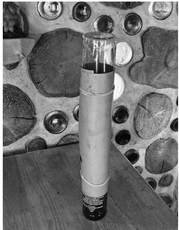
9.12: Adjusting the length of the cylinder allows for bottle-ends from 16 to 24 inches in length.
