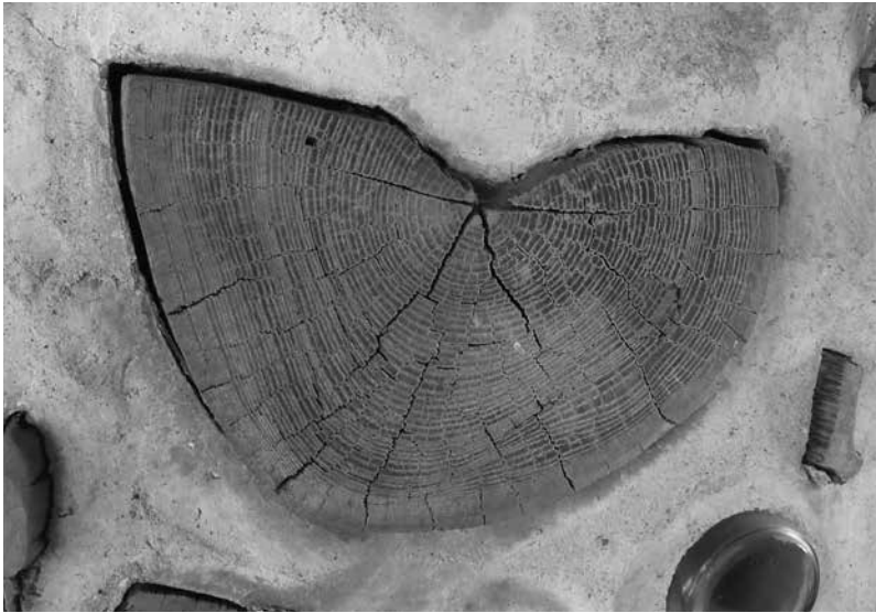
5.7: Radial shrinkage in this split hardwood log-end is seen clearly on the left outer edge. The top edge shrinking is tangential shrinkage.
