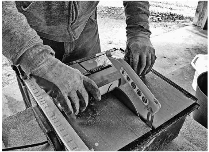
9.9: Slate and tile saw used for cutting bottle-ends.
