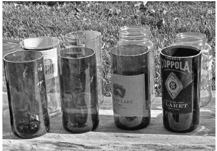
9.10: Bottles have been cut into tumblers (except for two jars, useful as they are), and are drying in the sun. Keep your pairs together throughout the process. Remove labels if they come off easily during the washing process. At the very least, remove any label material within an inch of the end of the bottle, so that it does not show. A razor blade knife works well for this.
