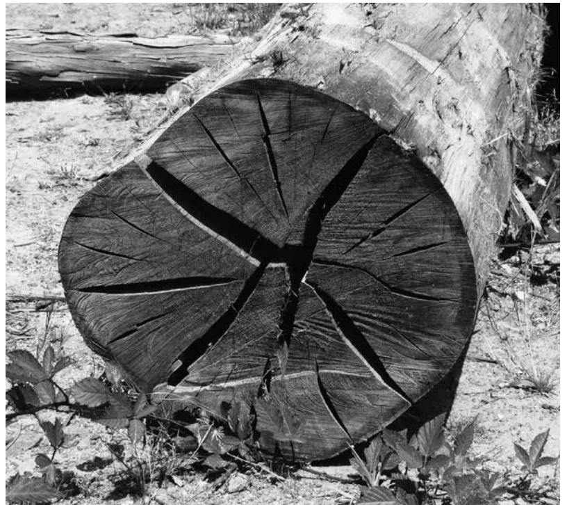
5.6: Eucalyptus does not seem to follow the “primary check” rule. It also doesn’t split very well. In fairness, there are more than a hundred varieties, and some might perform differently from others.
