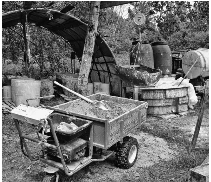
5.15: Bruce Kilgore's "production line" mixing area. Note the scales.
