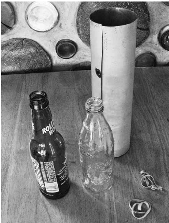
9.11: A green and a clear bottle of the same diameter can be plugged into a flexible cylinder and held fast with two strong elastic bands.
