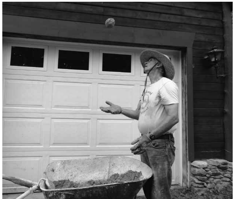
8.4: Test frequently until you know your mortar. Do the "snowball test."
