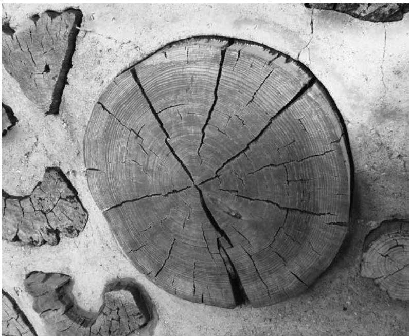
5.8: This hardwood log-end shows radial shrinkage around its perimeter, as well as tangential shrinkage in the form of checking.
