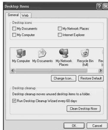
FIGURE 7.3 Clicking the Customize Desktop button produces the Desktop Items properties sheet with a number of customization options on the General and Web tabs.
