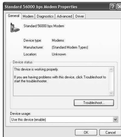
FIGURE 25.6 The Property sheet for a modem allows you to configure specific options for the modem.
