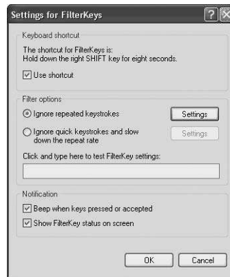
FIGURE 5.5 Use the Setting for FilterKeys dialog box to make Windows XP ignore repeated keystrokes or to change the rate at which a character is repeated when a key is held down.
