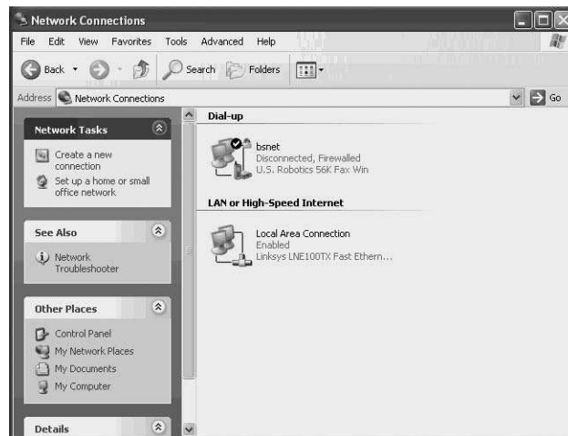
FIGURE 24.4 The Network Connections dialog box shows you the Local Area Connection entry created for your network card.
