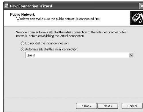
FIGURE 25.24 Select whether to automatically dial a connection when you use the VPN.
