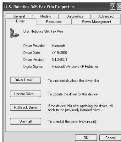
FIGURE 23.8 Use the Roll Back Driver button on a device's properties pages to return to a previous version of the driver.
