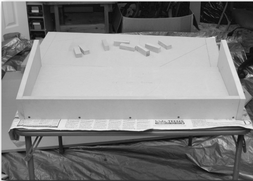
FIGURE 2-26: Partially assembled control panel box, with mounting pieces and marked top in the background.
