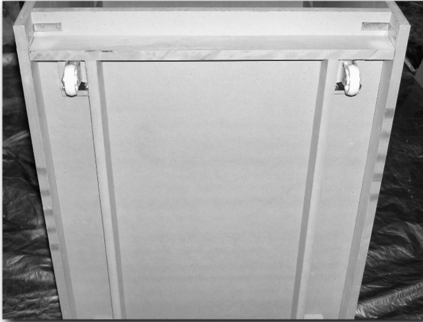
FIGURE 2-15: Installing the L-brackets on the underside.
