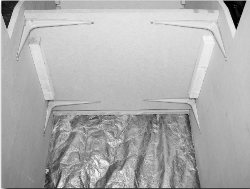
FIGURE 2-22: The monitor shelf (from underneath), mounted and ready for use.
