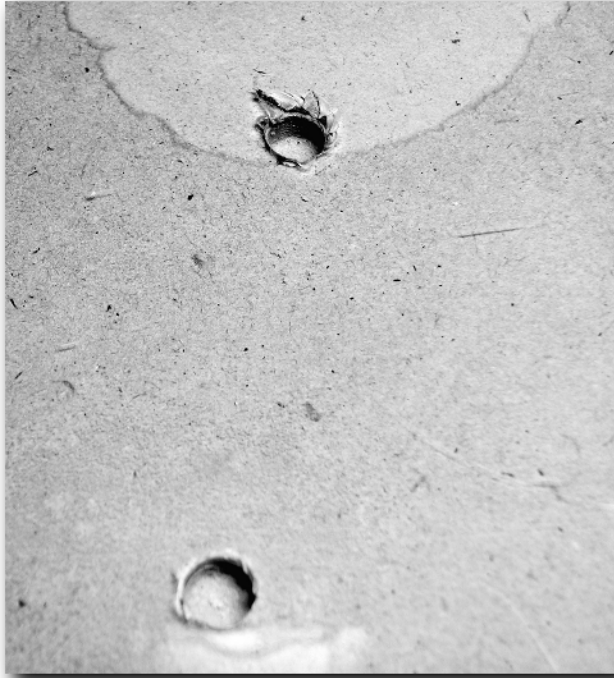
FIGURE 15-10: Below, slowly drilled hole. Above, cracked hole.
