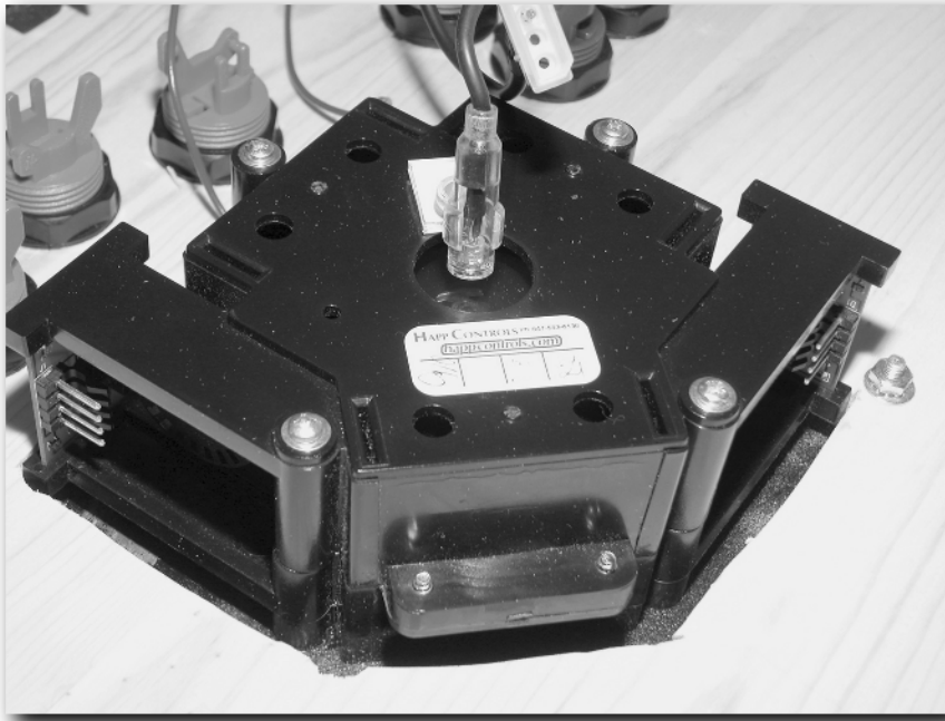
FIGURE 15-15: Happ Controls trackball with super-bright LED attached. Used by permission of Happ Controls.
