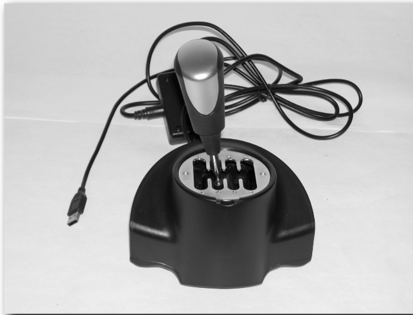
FIGURE 5-5: The Act-Labs GPL USB shifter in native eight-position mode.
