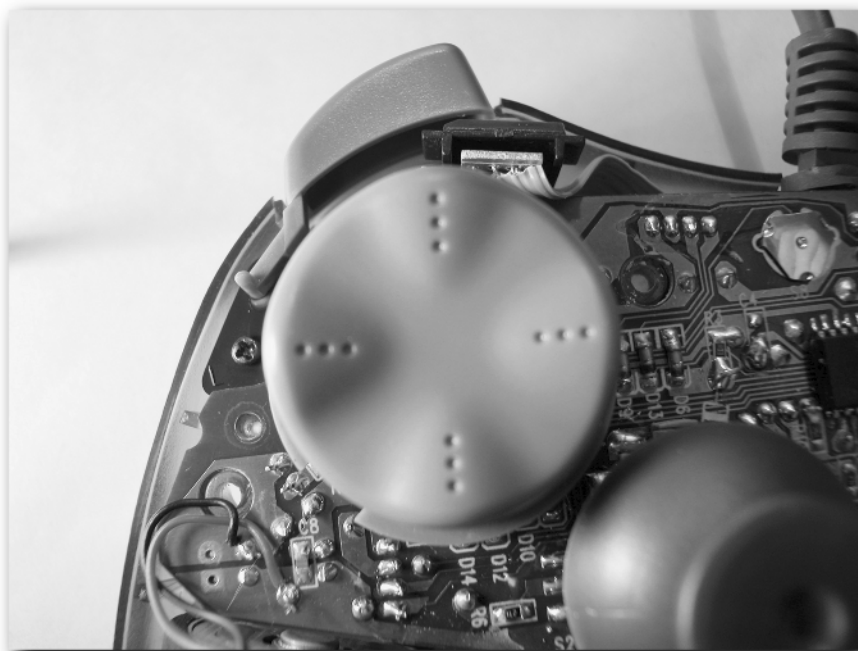
FIGURE 10-5: A partially disassembled gamepad showing the directional pad.
