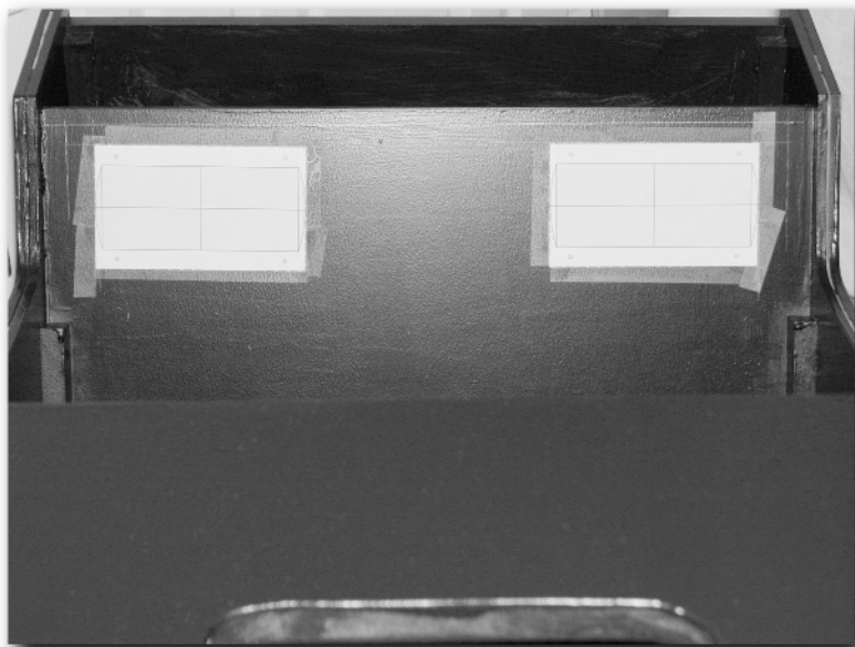
FIGURE 11-6: Underside of speaker shelf with templates in place.
