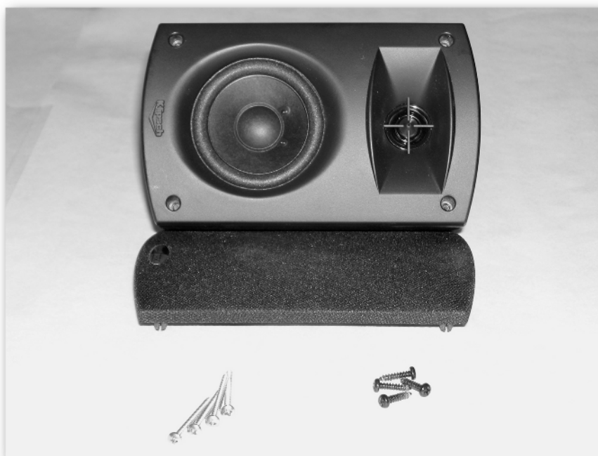
FIGURE 11-8: Klipsch ProMedia 2.1 speaker with cover and screws removed. Replacement screws are on the left; original screws are on the right.
