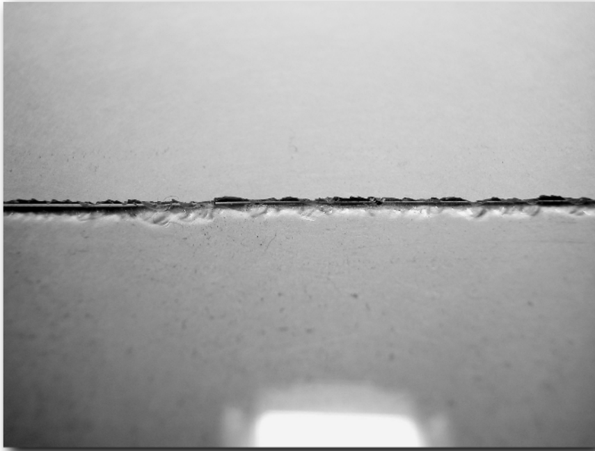
FIGURE 15-6: This Plexiglas was improperly cut, causing a rough edge.
