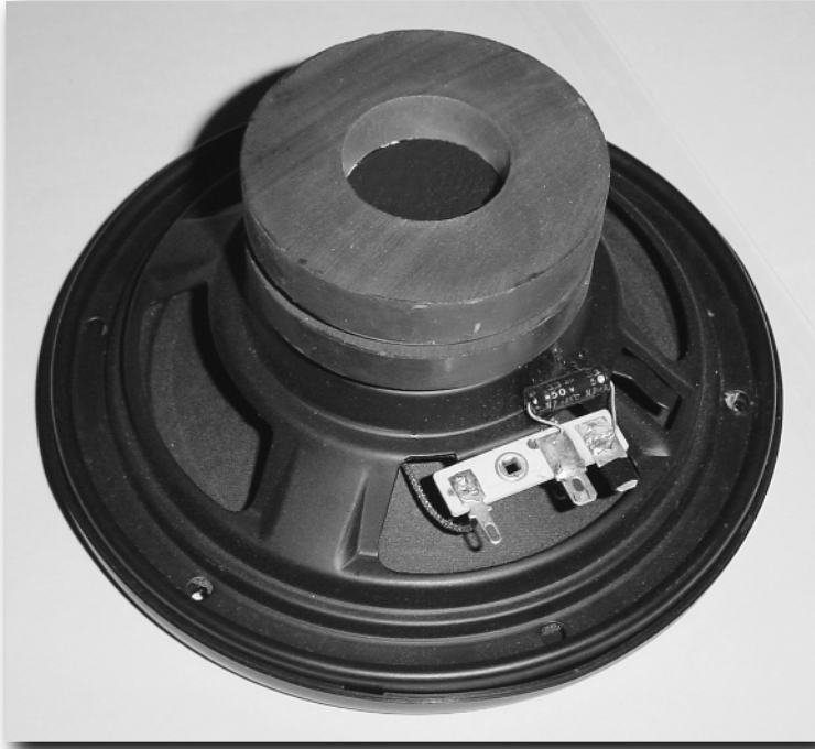
FIGURE 11-3: A bucking magnet attached to a car stereo speaker.
