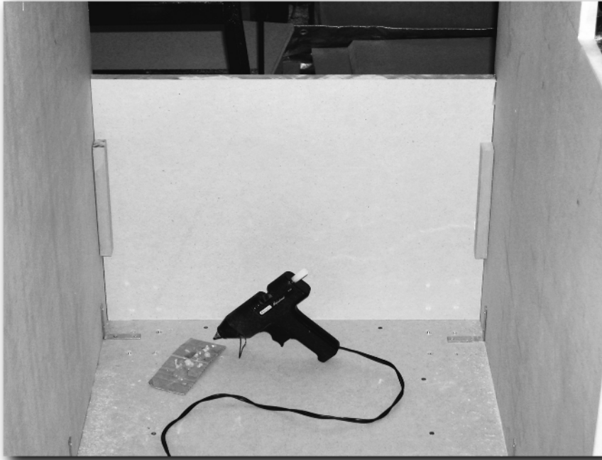
FIGURE 2-17: The cabinet back bottom section securely fastened into place.
