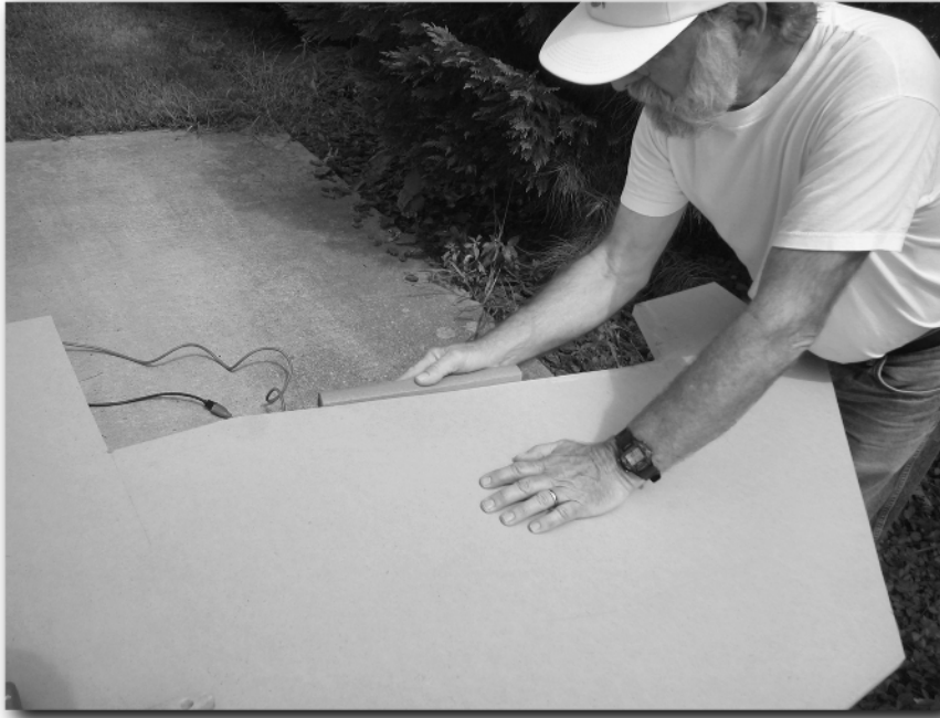
FIGURE 2-9: The sanding block makes quick work of a small variance in this cut.
