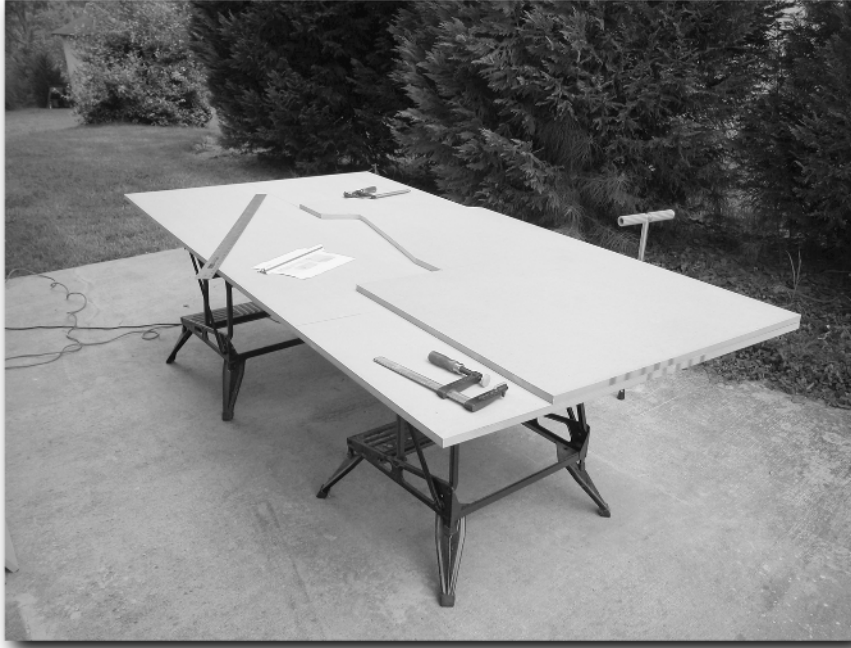
FIGURE 2-8: Using one cabinet side as a template for the second.
