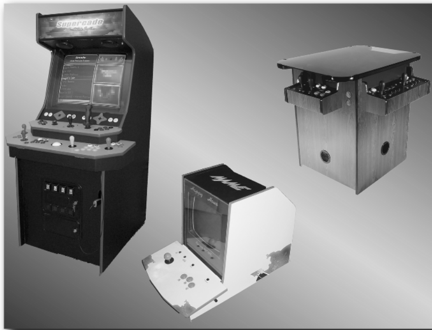
FIGURE 1-2: A variety of different arcade cabinets. From left: Upright, countertop, and cocktail. Photo courtesy of Jeffrey Allen, Oscar Controls, and Game Cabinets, Inc., respectively.
