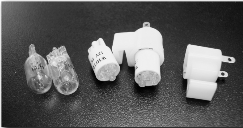
FIGURE 15-18: Regular light bulbs and the three LED super-bright cluster replacements. Used by permission of Happ Controls.
