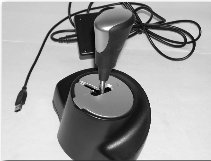
FIGURE 5-6: The same shifter with the hi/lo overlay plate installed.
