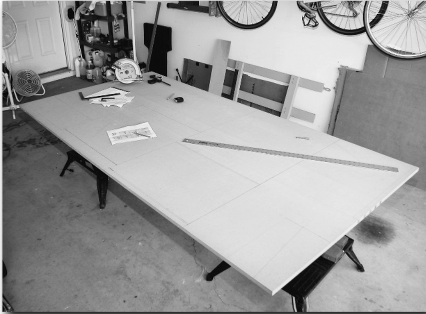
FIGURE 2-4: Drawing out the first sheet of wood.
