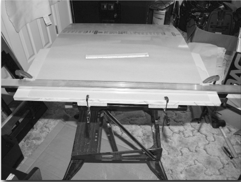
FIGURE 15-7: Straight-edge, Plexiglas, and wood sandwich.
