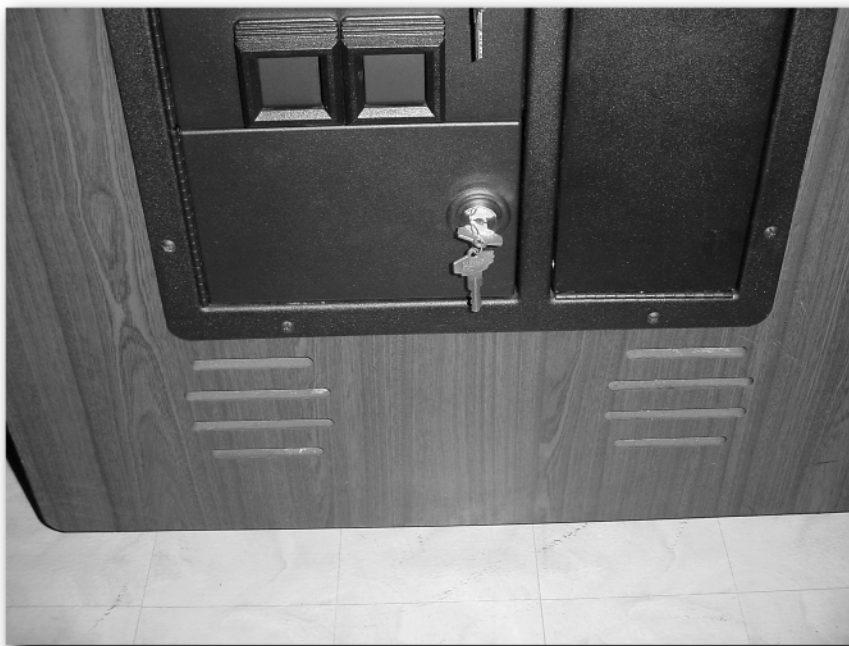
FIGURE 11-4: Routed speaker cutouts on a cocktail cabinet.
