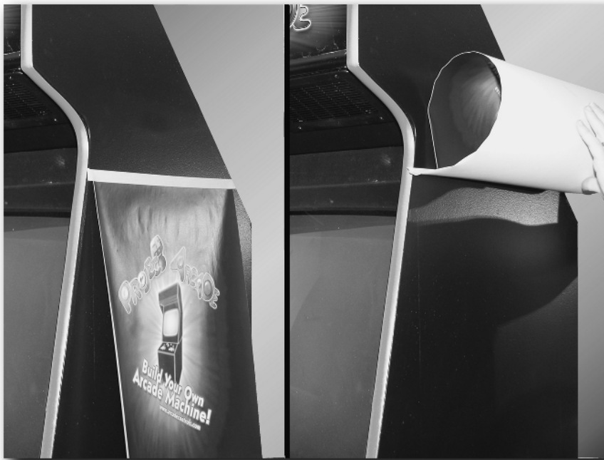
FIGURE 15-4: Applying the artwork.
