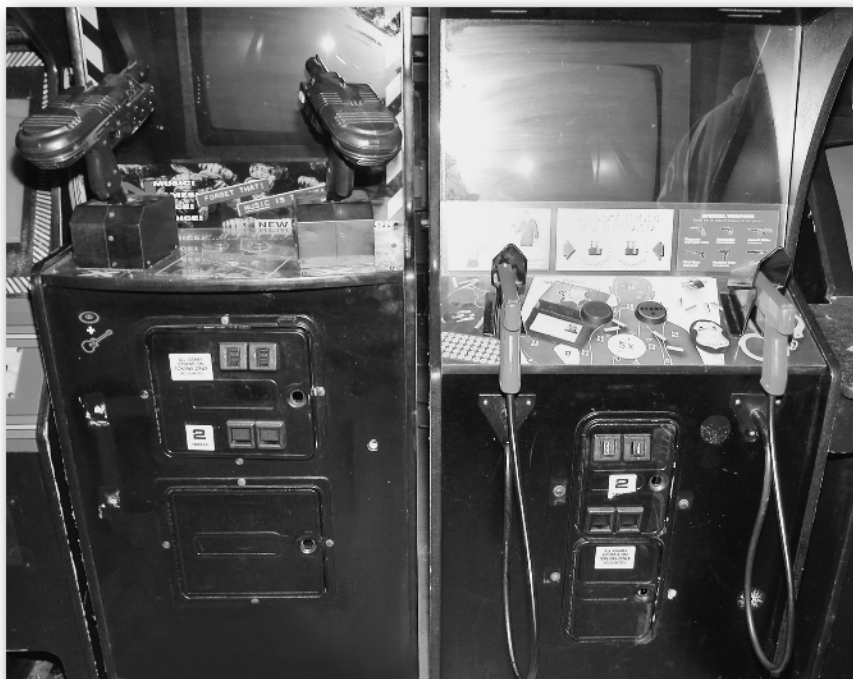
FIGURE 5-10: Fixed positional guns (left); one employing light guns (right).
