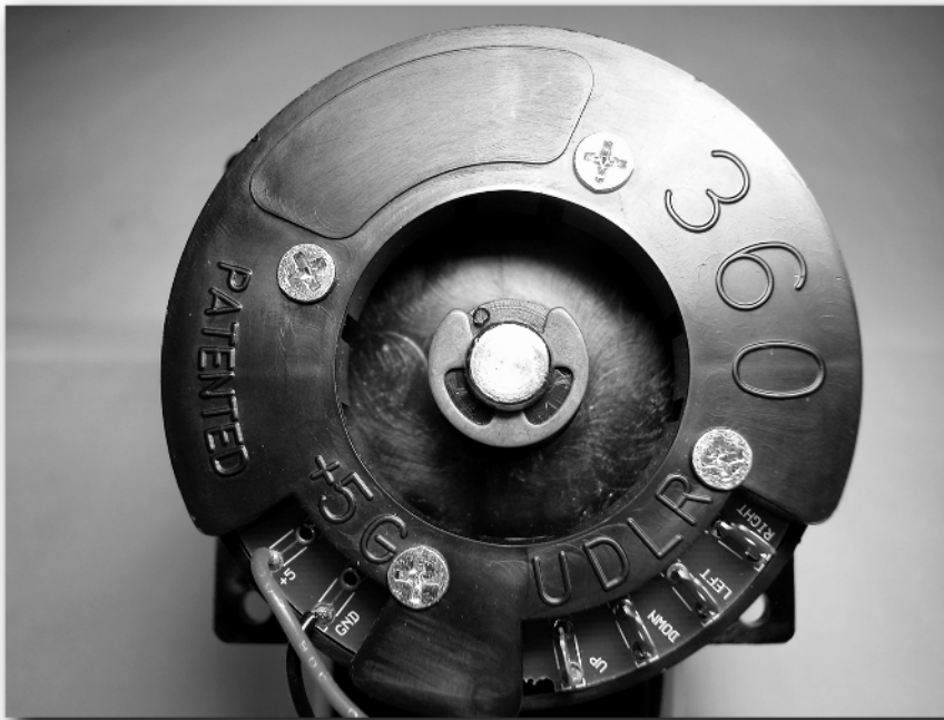
FIGURE 7-13: The labeled underside of a Happ Controls Perfect 360 joystick.
