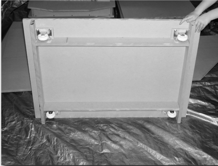
FIGURE 2-12: The assembled cabinet base with casters.
