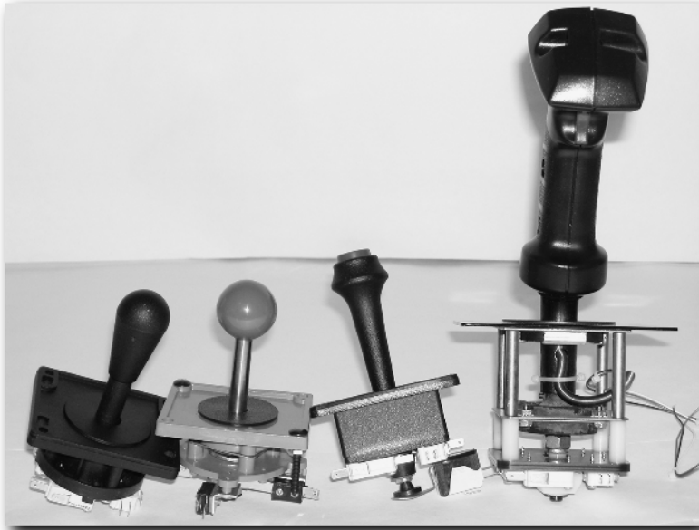
FIGURE 3-12: From left to right, bat-shaped, ball-shaped, flare-type, and trigger-grip handles.
