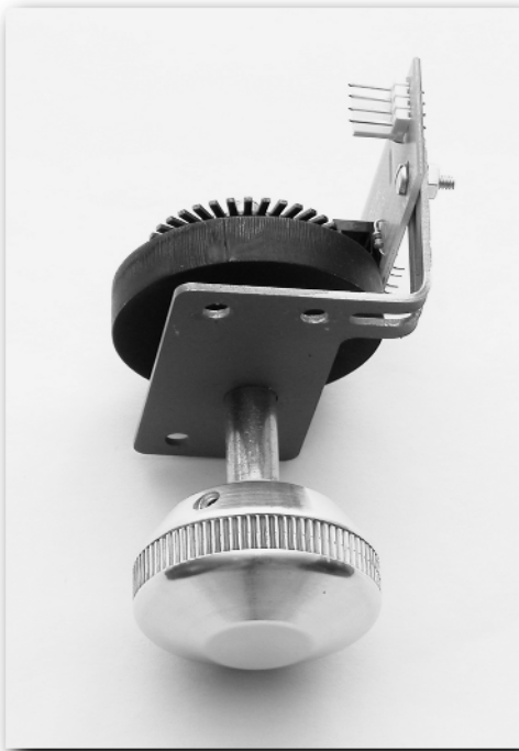
FIGURE 4-5: Model 3 spinner with Discs of Tron replica knob, no mounting plate.
