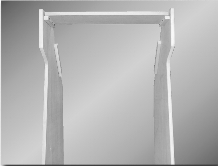
FIGURE 2-18: The cabinet top securely mounted into place.
