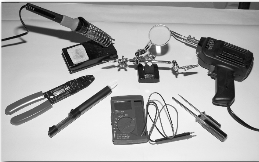
FIGURE 7-4: Most of the tools you're likely to need for wiring. Clockwise from upper left: Soldering iron in soldering station, extra hands, soldering gun, screwdrivers, multimeter, solder-removal tool, and crimping tool.
