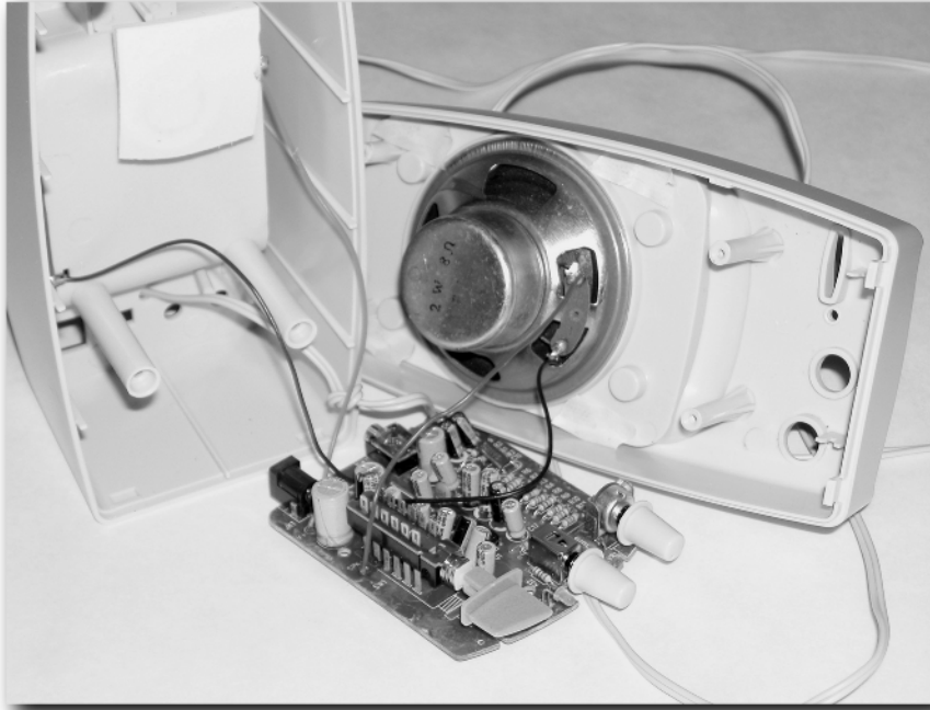
FIGURE 11-2: Amplifier from generic PC stereo speakers.
