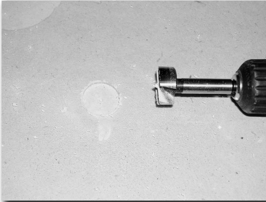
FIGURE 15-11: A smoothly cut button hole next to the forstner bit.
