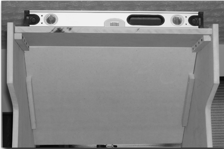
FIGURE 2-20: The cabinet back angled section in place (speaker shelf removed for photo).
