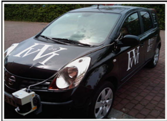
Fig. 1 Intelligent vehicle based on visual information (IVVI) 2.0
