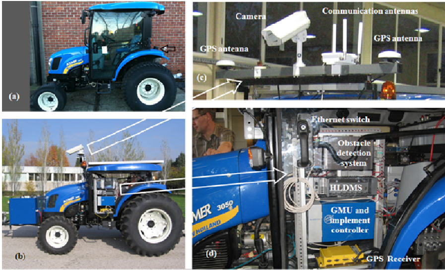
Fig. 4. (a) Initial commercial tractor; (b) final RHEA GMU; (c) external equipment onboard the GMUs and (d) internal equipment distribution inside the GMU's cabin
