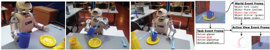
Fig. 10. Description for experiment B in the knowledge base scenario. At the beginning the task can be started by either picking the cup or the spoon. (left) The HOAP-3 robot start the task by grasping the blue cup . (center-left) With the cup and the spoon in its hands the robot performs the action skill to put the spoon inside the cup. (center-right) Finally, the HOAP-3 robot places the blue cup on the saucer plate. (right) State of the knowledge base at some step during execution. From the Task and World Events the Active View Event is built to drive the action execution.
