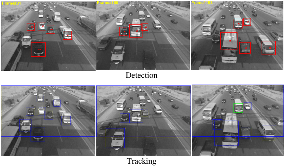
Fig. 4. Heavy flow: Top row shows detected targets (red), Bottom row shows tracked targets (blue) and first time detection (green). ROI controls tracked targets removal.
