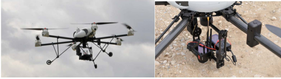
Fig. 2. RHEA drone in flight with a detail of the cameras mounting
