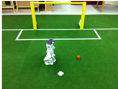
Fig. 3. Experimental setup. The environment is the real SSL field and the robot is equipped with a pattern in order to be detected by a ground truth system.
