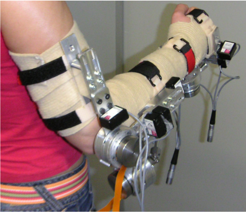
Fig. 1. Assistive Robotic device for tremor reduction (WOTAS, Wearable Orthosis for Tremor Assessment and Suppression)
