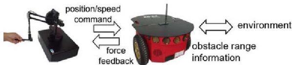
Fig. 3. Teleoperation is one of the most common way for wheeled mobile robots. In this case, extracted from [58], a Pioneer 3-DX robot is teleoperated by a Phantom Premium haptic device.
