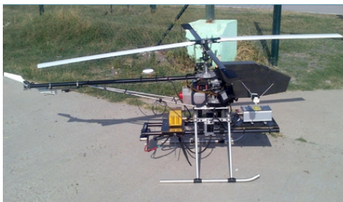
Fig. 1. (Right) RUAV platform with all the avionics to collect the frequency sweep data. (Left) CB-5000 main characteristics.
