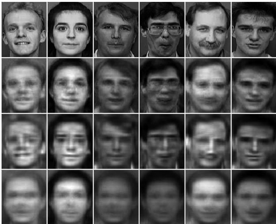
Fig. 13.7 Tensor factorization vs. matrix factorization on facial data. Six randomly chosen images from 400 of ORL dataset. From top to bottom: original images, their rank-8 truncated SVD approximation, their rank-142 nonnegative tensor approximation (150 RRI iterations) and their rank-8 nonnegative matrix approximation (150 RRI iterations)
