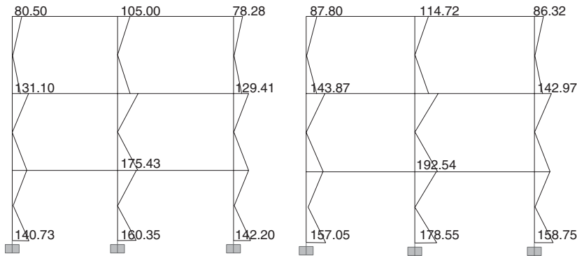
Figure 4.33 Bending moments (in kNm) computed through response spectral analyses using two different modal combinations for three-storey frame: square root of the sum of the squares ( left ) and complete quadratic combination ( right )
