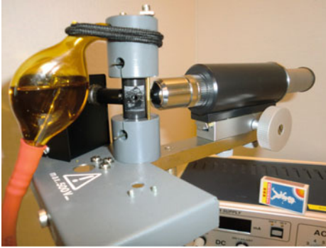
Fig. 5.4 The Millikan apparatus, student version by PHYWE. The oil drops are illuminated and observed by the telescope. Using a built-in distance scale the velocity of an oil drop may be determined through a time measurement. The voltage over the capacitor plates is established by means of the pins on the picture
