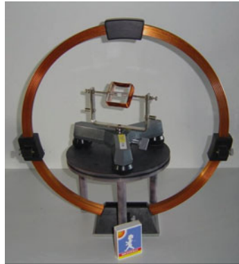
Fig. 2.13 Two closed conductors utilized for investigation of the induction effect. One of them is connected to a battery and the other to a current meter. The right-hand figure shows an example of an apparatus
