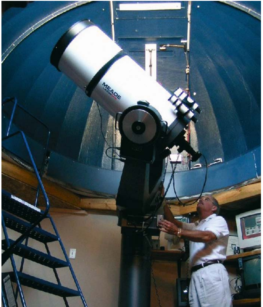
Figure 2.8. An especially solid fork mounting supplied with premium-quality Schmidt-Cassegrain telescopes, outfitted nicely with electronic slow-motion controls, clock drive, and other refinements. Polar axis alignment is accomplished using a special wedge designed for the latitude of the observer. (Credit: Brian Sherrod, Arkansas Sky Observatory.)
