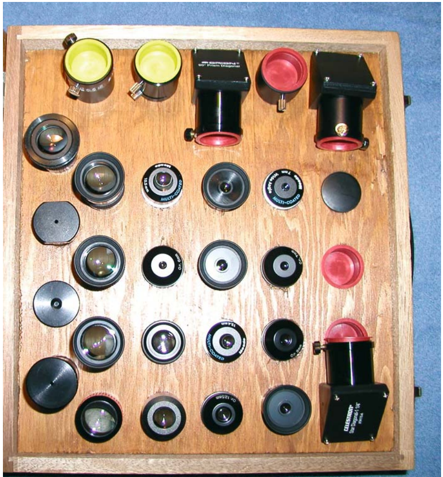
Figure 2.10. A good collection of eyepieces for planetary viewing in a homemade dust-proof wooden case. Observers should avoid using foam-lined cases, because foam deteriorates with time and can damage eyepieces and accessories. (Credit: Julius L. Benton, Jr.)
