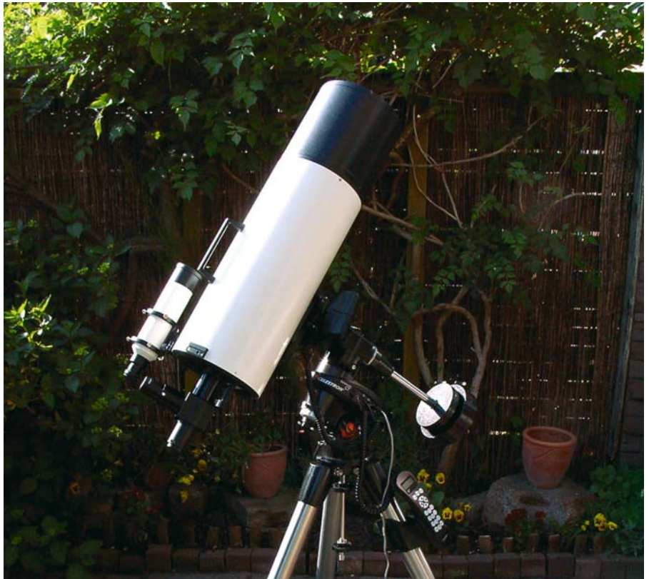
Figure 2.6. Maksutov–Cassegrains, such as this very fine 18.0-cm (7.1-in) model, are powerful long focal length ( f/10 to f/13 ) instruments in a relatively small package for planetary work. Their collimation usually remains stable even after considerable handling, much like refractors. (Credit: Jan Adelaar; ALPO Saturn Section.)
