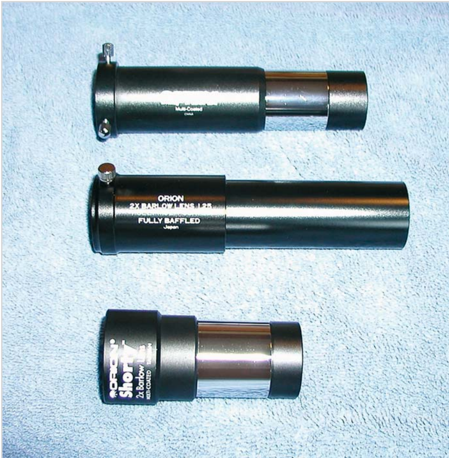
Figure 2.12. Several achromatic Barlow lenses sporting magnifications between 2× and 3×. They conveniently expand the magnification ranges of a given set of eyepieces. (Credit: Julius L. Benton, Jr.)
