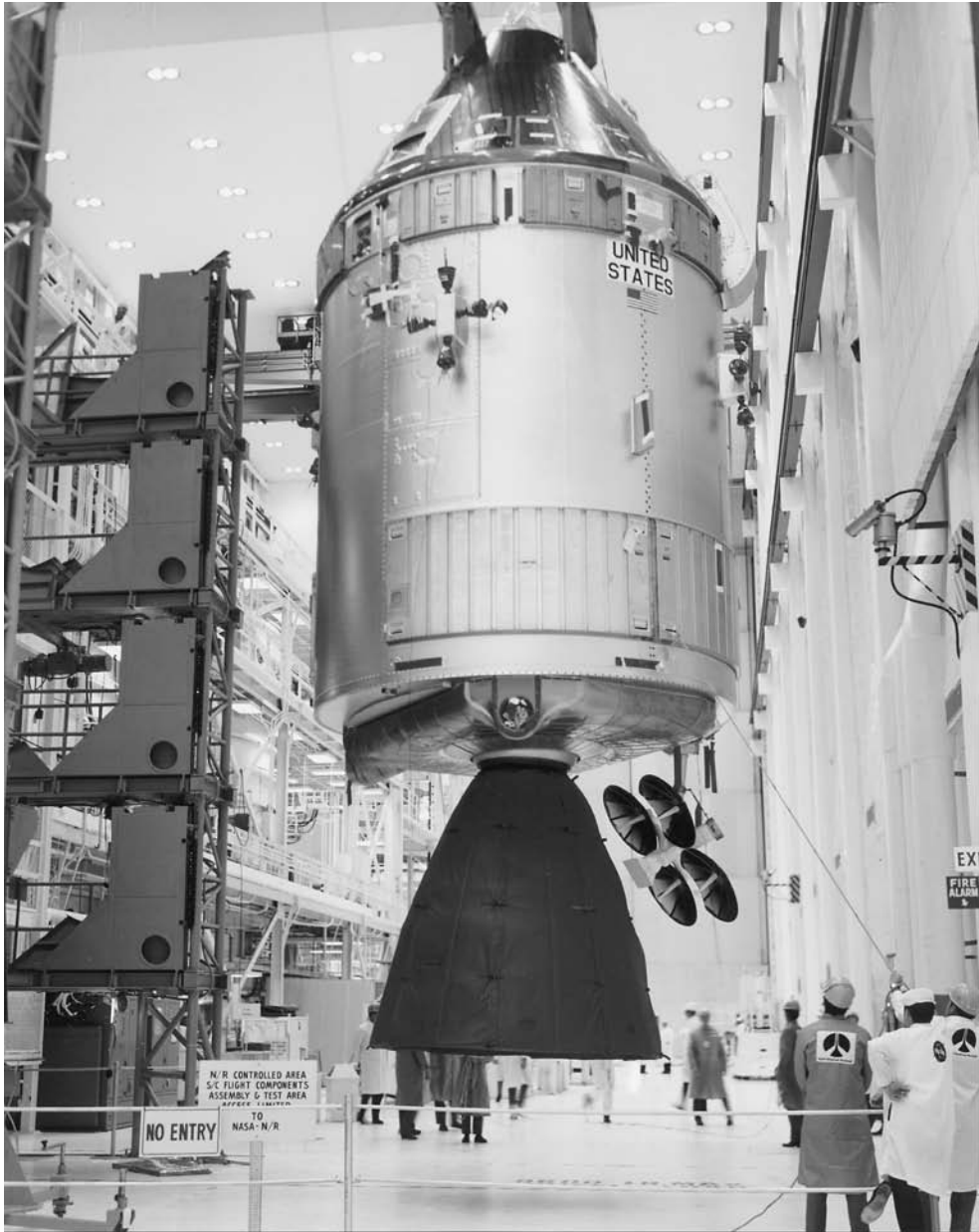
Command service module 109, which would become part of Apollo 13, hangs in a clean room before being lifted to its position atop the Saturn V. No one realized that there was a damaged part deep within the service module that would disrupt the mission.
