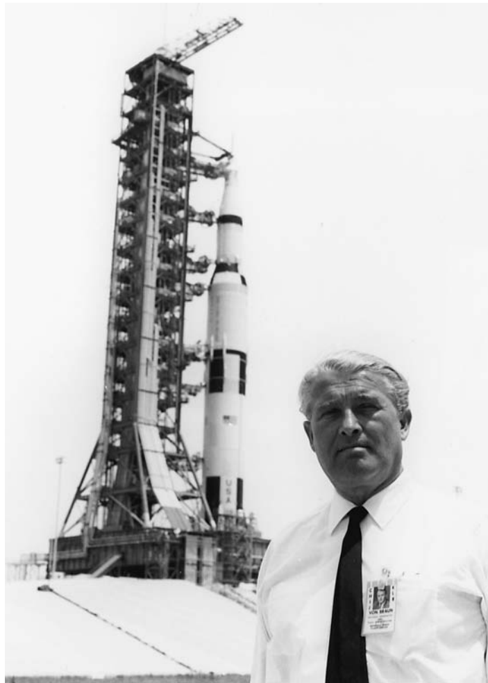
Wernher von Braun stands in front of the Saturn V rocket. The 363-foot-tall three-stage rocket provided enough power to shoot the Apollo astronauts out of Earth’s gravitational pull and toward the moon.
